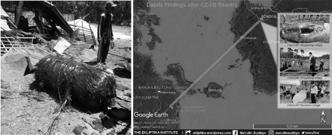
Figure 5: Left: Carbon-fibre-wrapped pressure tank of a Falcon 9 upper stage recovered after uncontrolled re-entry on Java [11] Right: Debris possibly associated with this space debris was found after the CZ-5B re-entry over Indonesia in early August 2022. 3 Debris found by locals in Sanggau regency (near the Indonesian-Malaysian border) [12]
