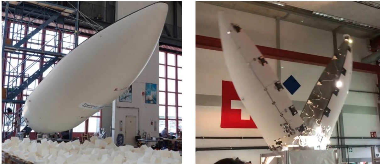
Figure 9: Full-scale testing; left: demonstration test of hinged jettison system for a Ø2.6m MLV PLF; right: demonstration test of the full separation and jettison system for a Ø1.5m SLV PLF
