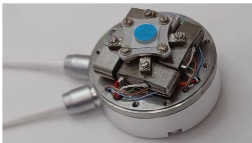
Figure 16: Miniature FSM (with a protection layer on mirror)
