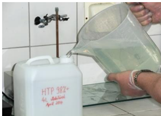
Fig. 2. Safe handling of 98% HTP at the laboratory of the Institute of Aviation in Warsaw.
