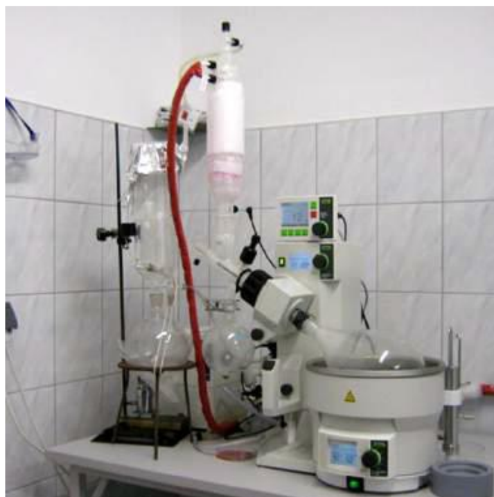
Fig.3. Laboratory test stand for purification on comercial H 2 O 2 to the purity of 99,99% [9].
