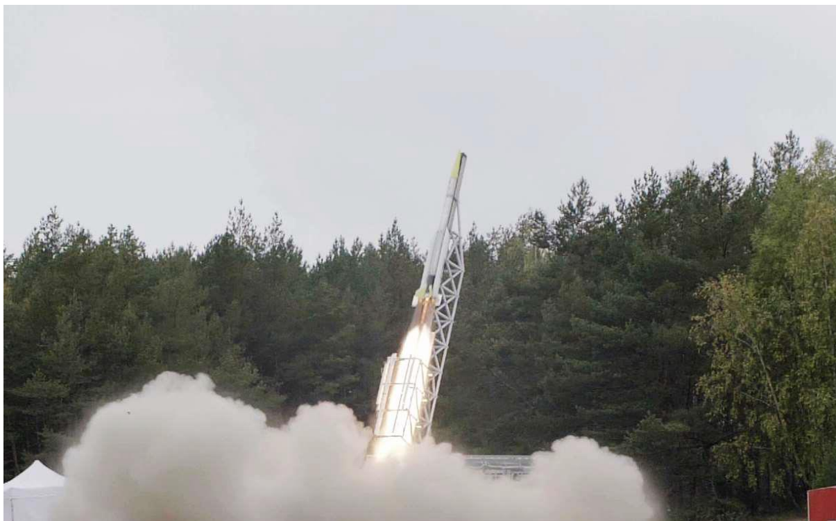
Fig. 8. Test launch of the “Bursztyn” rocket with main hybrid engine working on green propellants: a- initial stage just after ignition of both booster and main hybrid rocket engine, b- accelerated rocket on the launch pod [26].
