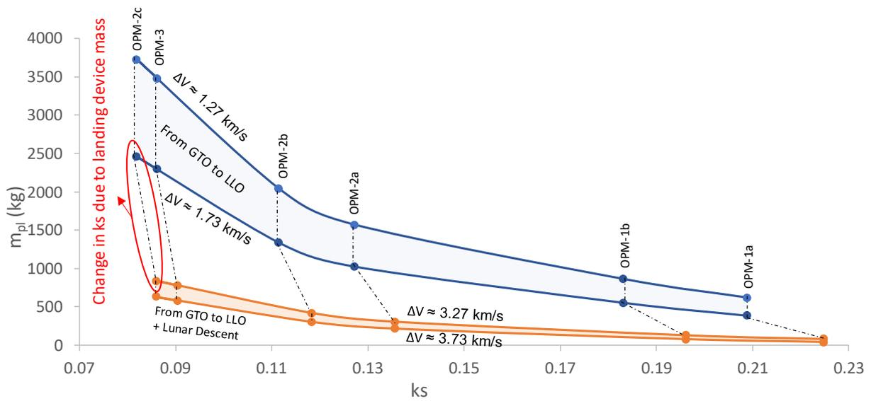
Figure 10: Payload mass vs structural efficiency, lunar shuttle and lunar lander missions with Ariane 6-2
