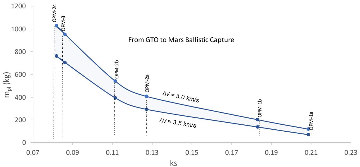
Figure 12: Payload mass vs structural efficiency, Mars missions with Ariane 6-2
