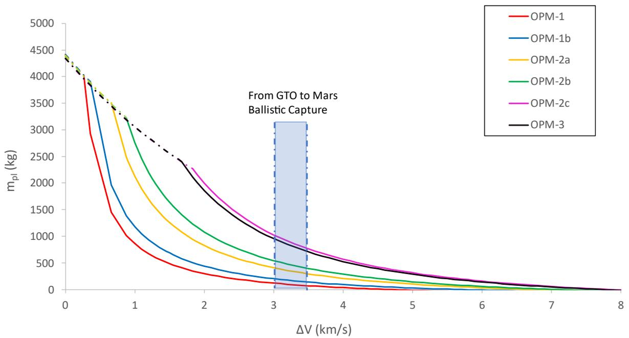
Figure 11: Payload mass vs  $\Delta V$ , Mars missions with Ariane 6-2
