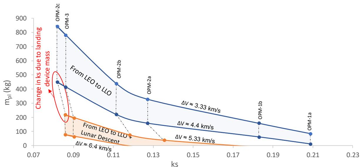
Figure 7: Payload mass vs structural efficiency, lunar shuttle and lunar lander missions with Vega C
