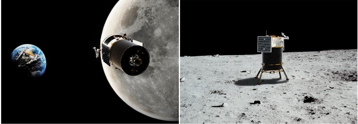
Figure 8: Use of Vertue OPM for lunar missions: lunar shuttle (left) and lunar lander (right).
