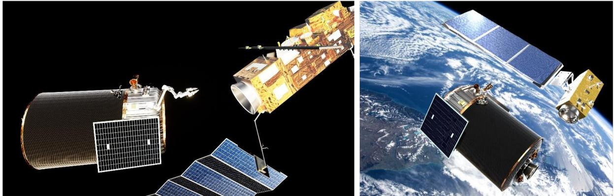
Figure 5: Vertue OPM performing IOS on ENVISAT satellite (left) and deploying a Sentinel-class Earth observation satellites (right).
