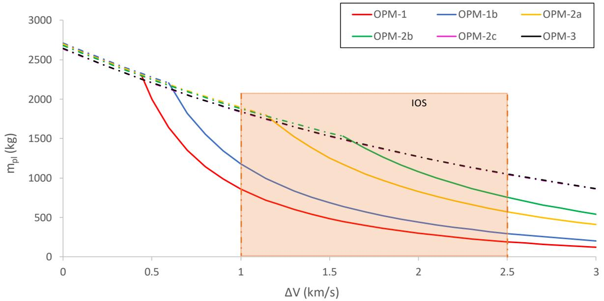
Figure 4: Payload mass vs  $\Delta V$ , IOS with Vega C
