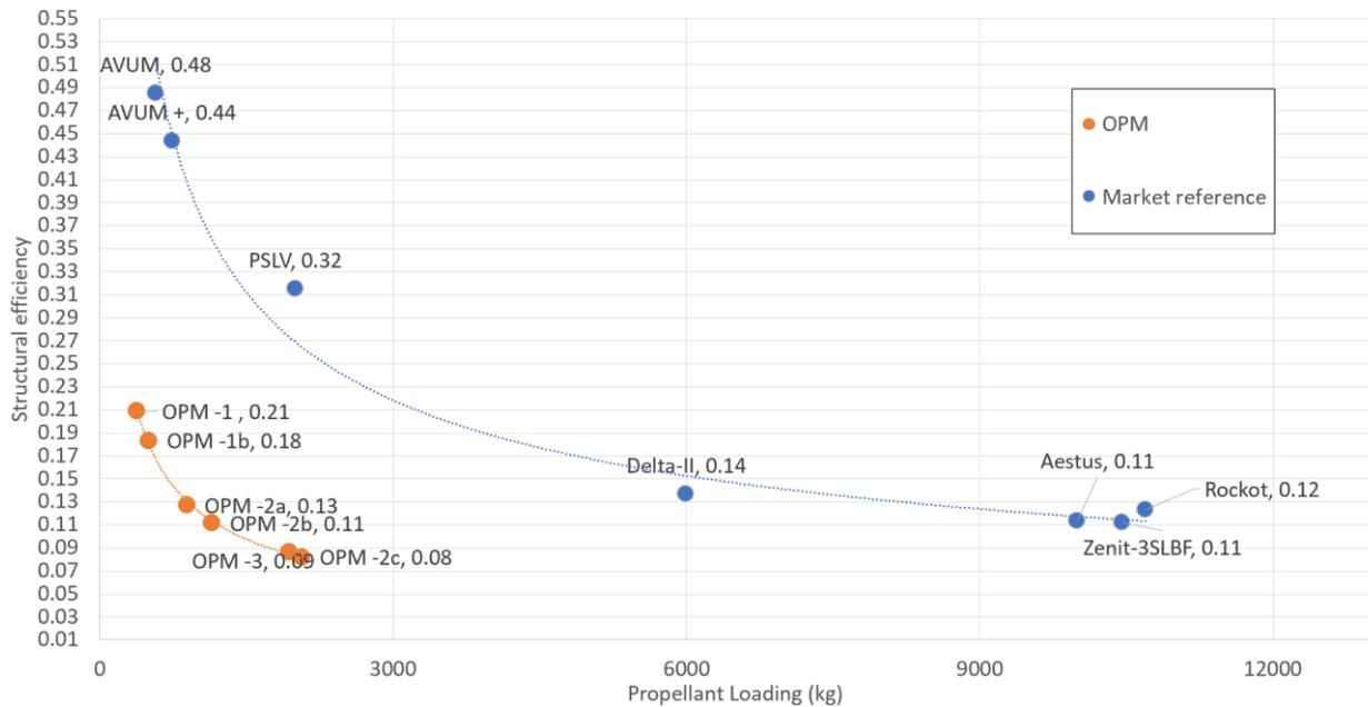
Figure 3: Structural efficiency of Vertue OPM compared to the state of the art.
