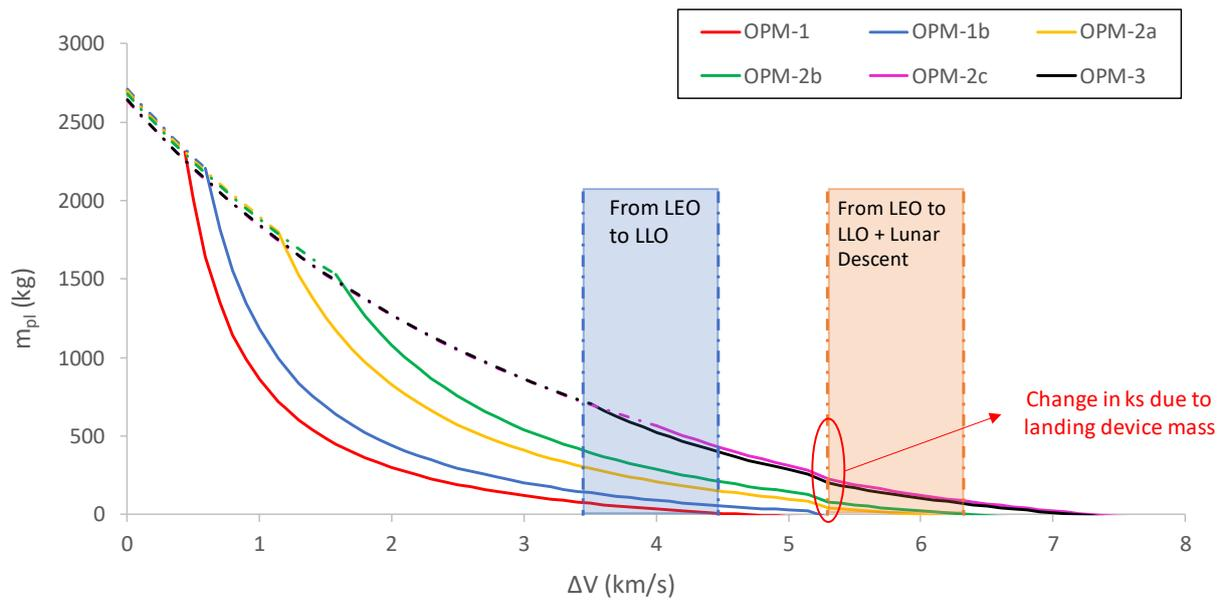
Figure 6: Payload mass vs  $\Delta V$ , lunar shuttle and lunar lander missions with Vega C
