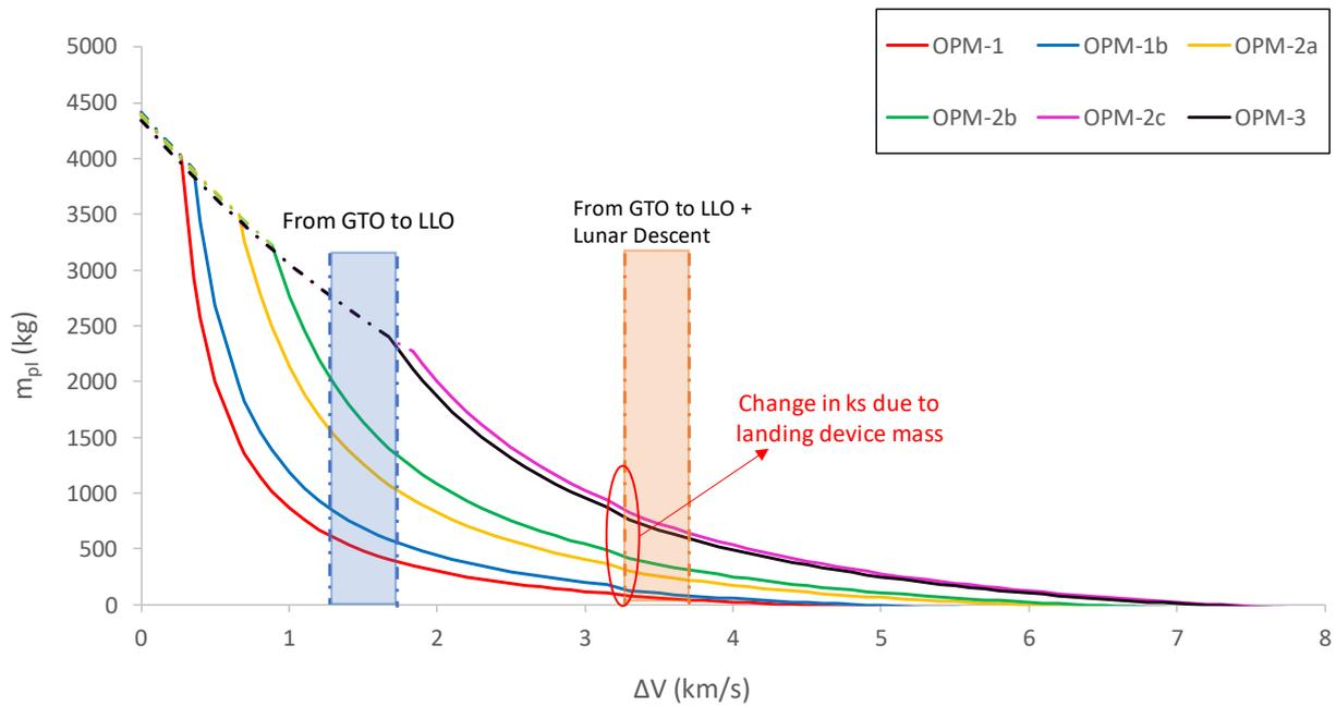
Figure 9: Payload mass vs  $\Delta V$ , lunar shuttle and lunar lander missions with Ariane 6-2
