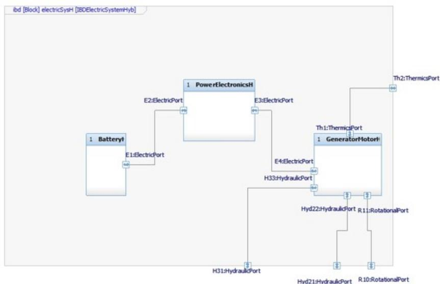
Figure 7: Extension of the electrical system
