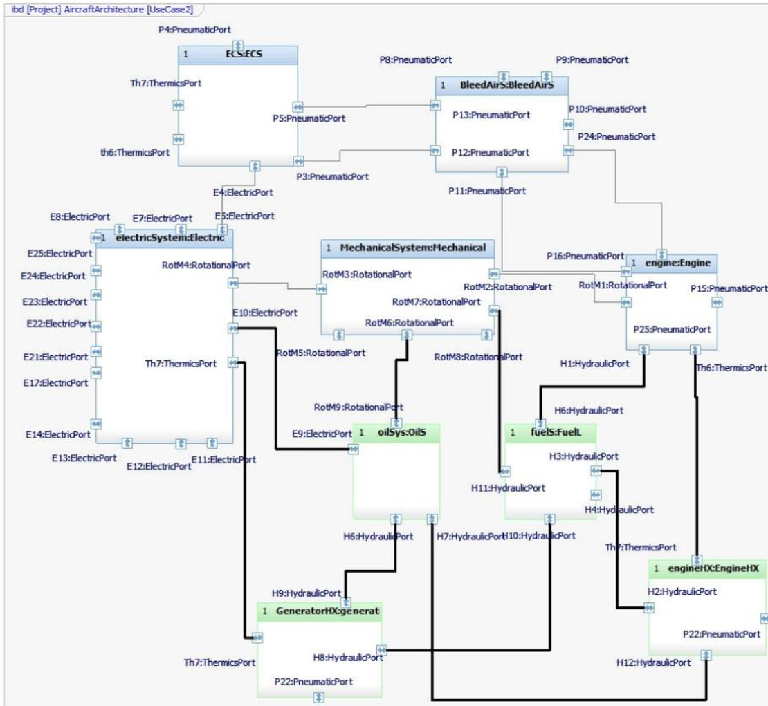
Figure 5: Extension of the use case with engine and generator cooling loops
