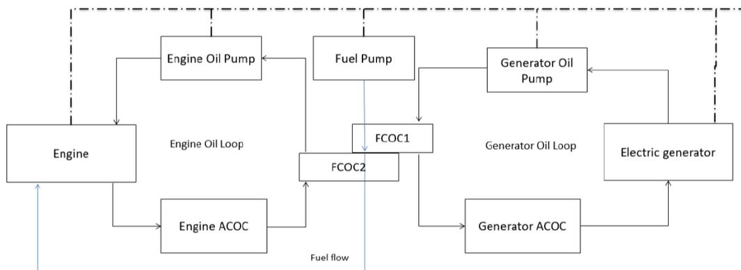
Figure 6: Proposed structure of thermal oil loop integration with Engine/Generator
