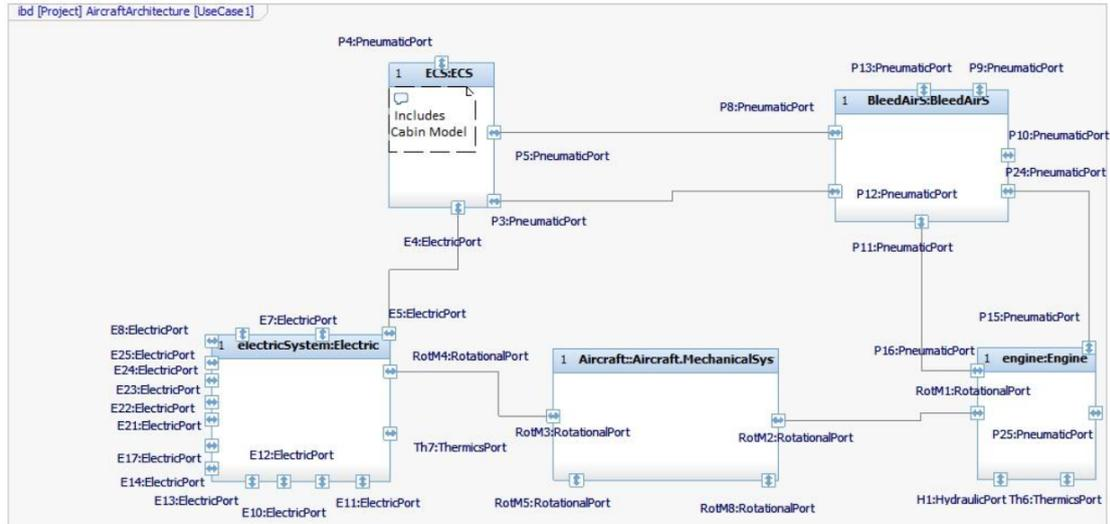
Figure 3: ECS, electrical system and engine integration use case
