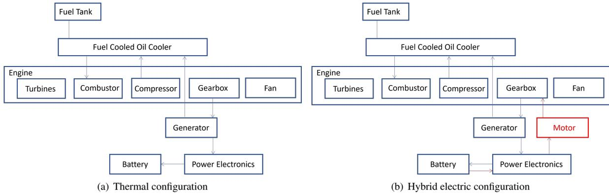
Figure 8: Extension of the existing thermal platform to a hybrid electric platform
