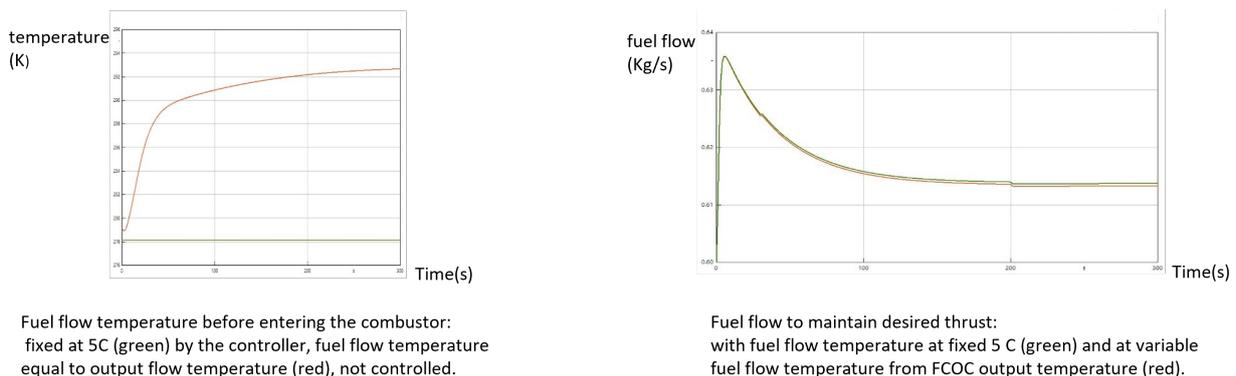
Figure 4: Thermal oil loop integration simulation
