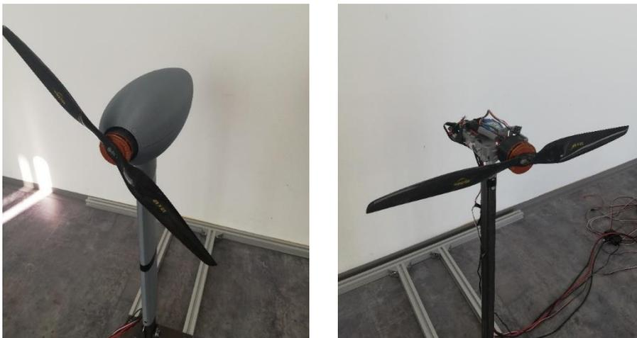
Figure 9 : The test rig, with and w/o fairing
