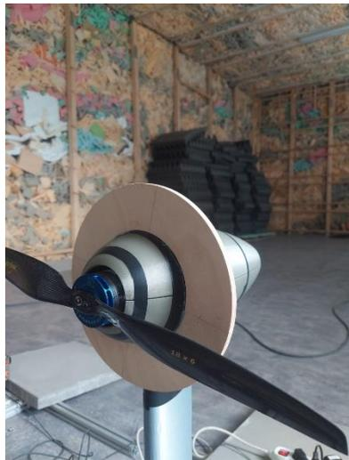
Figure 11 : Installation of forward, 25% clogging ring with 18x6 propeller
