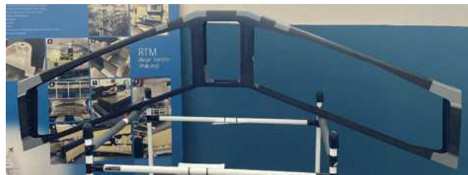
Figure 8. HTP Torsion Box RTM
