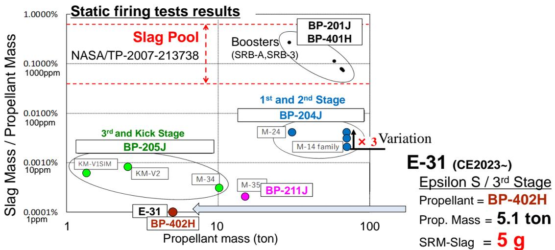
Figure 16: Updated mass ratio of alumina slag to propellant in major Japanese solid rocket motors.
