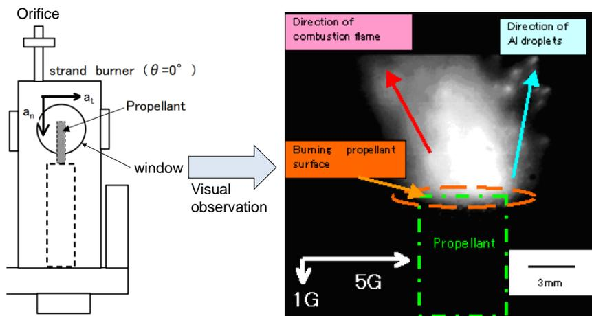
Figure 1: A photograph of flight of aluminum particles in centrifugal acceleration field [4]
