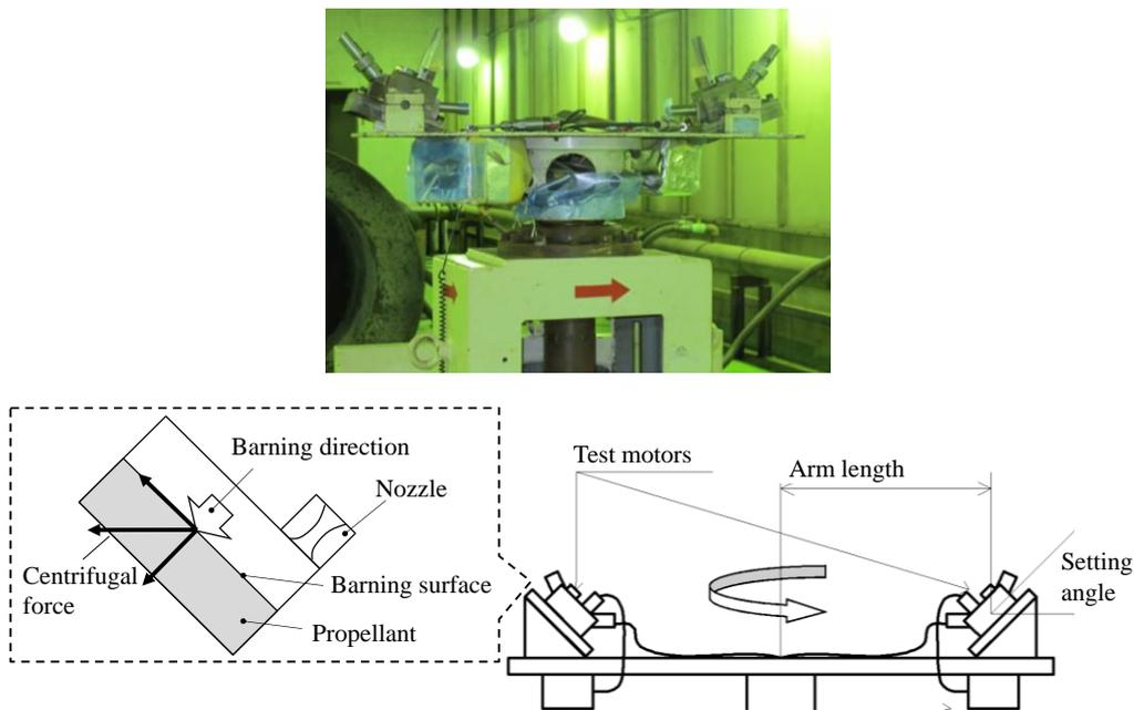
Figure 3: Schematic diagram of a small spin test stand
