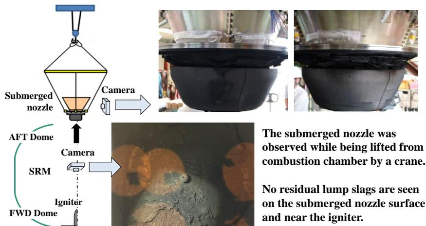
Figure 13: Image of the inside of E-31 after the firing test.
