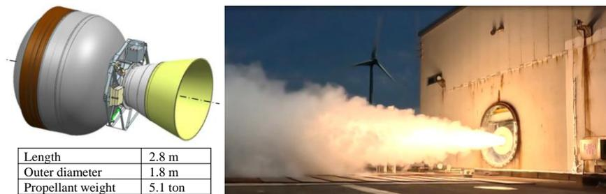
Figure 12: Image of the E-31 firing test situation.
