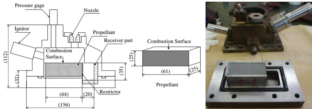
Figure 4: Small size test motor
