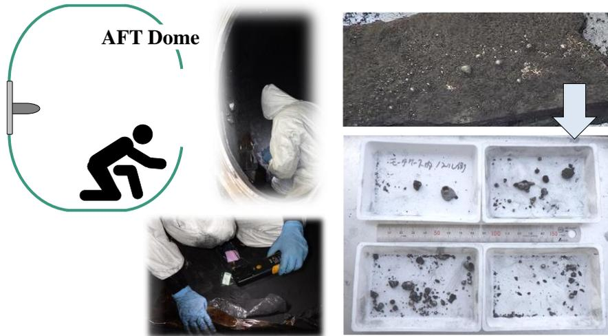
Figure 14: Collecting work of residual slag inside E-31 motor case.
