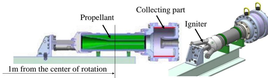
Figure 6: Test equipment
