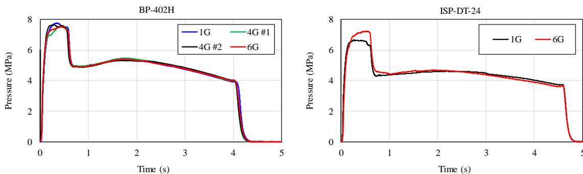
Figure 9: Combustion pressure results (left: BP-204H, right: ISP-DT-24)
