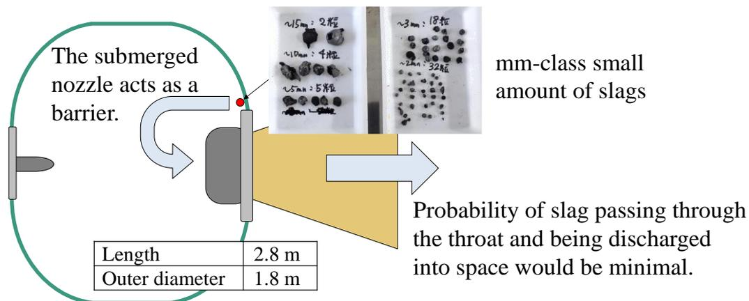
Figure 17: Positional relationship between slag accumulation region and submerged nozzle
