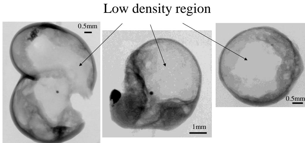
Figure 18: Results of X-ray computed tomography observations of slag particles
