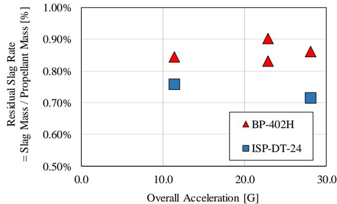
Figure 11: Overall acceleration sensitivity test results for residual slag rate
