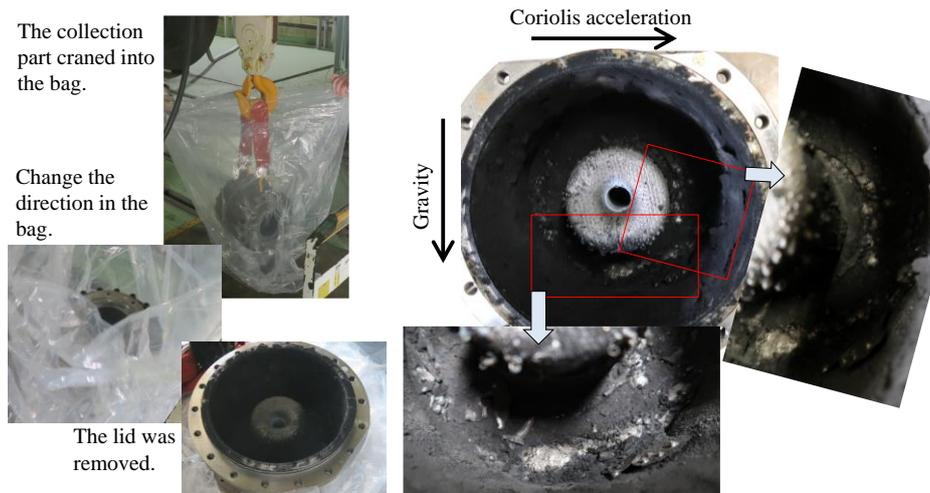
Figure 10: The accumulation of residual slag (1G, BP-204H)
