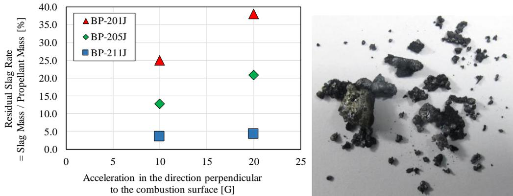
Figure 5: Acceleration sensitivity test results for residual slag rate and residual slag example
