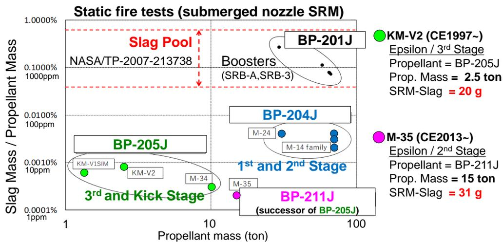
Figure 2: Mass ratio of alumina slag to propellant in major Japanese solid rocket motors [3]
