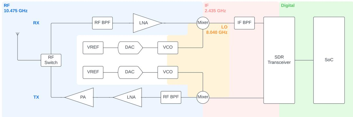
Figure 2: Block diagram of the transceiver architecture
