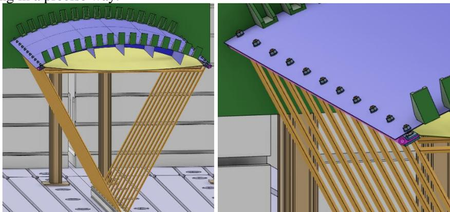
Figure 4: Bar structural assembly representing the omitted barrel segment (concept 1)
