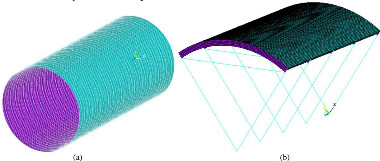
Figure 6: FE models of fuselage barrel (a) and test-rig concept 1 (b)
