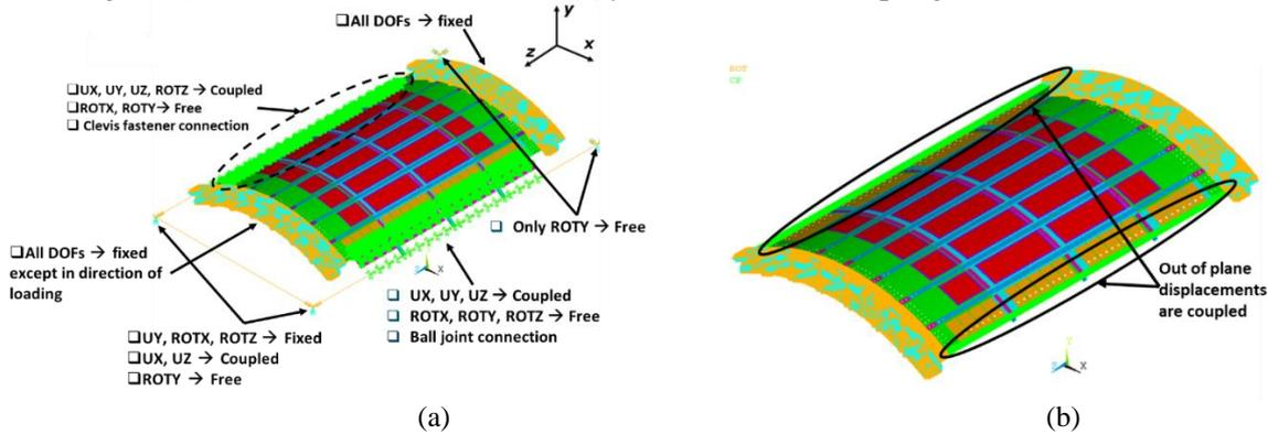
**Figure 9: The FE model of the panel inside the test-rig including BCs and couplings (a), the FE model of the panel with the simulated anti-buckling device (b)**
