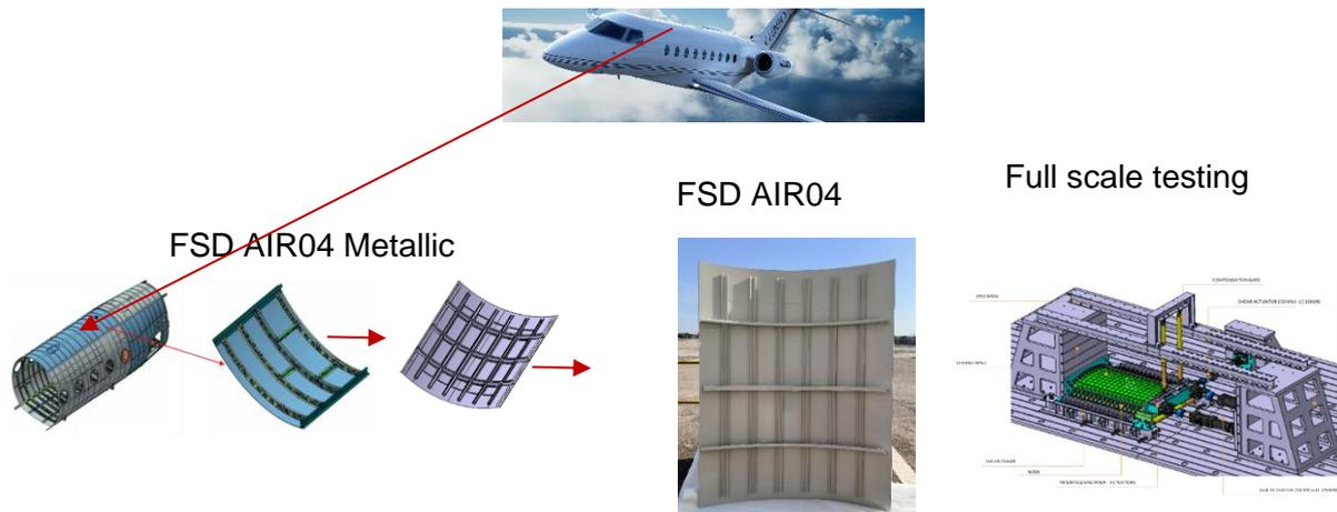
Figure 1: Scaling down process to focus on design elements and components of a fuselage [Clean Sky2 AIRFRAME FSD AIR04: Flagship Metallic fuselage demonstrator]
