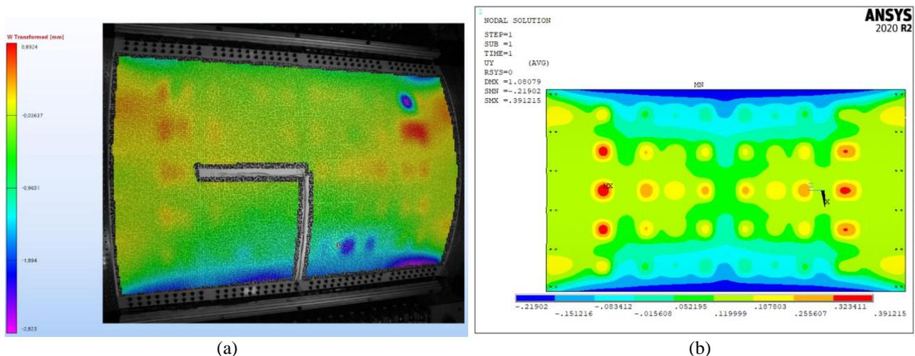
**Figure 10: Out-of-plane vertical displacement contours, DIC (a), FE (b)**
