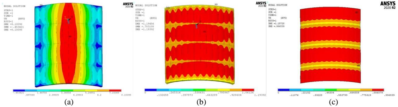
Figure 7: Radial displacements distributions for concept 1 panel (a), concept 2 panel (b) fuselage section (c)
