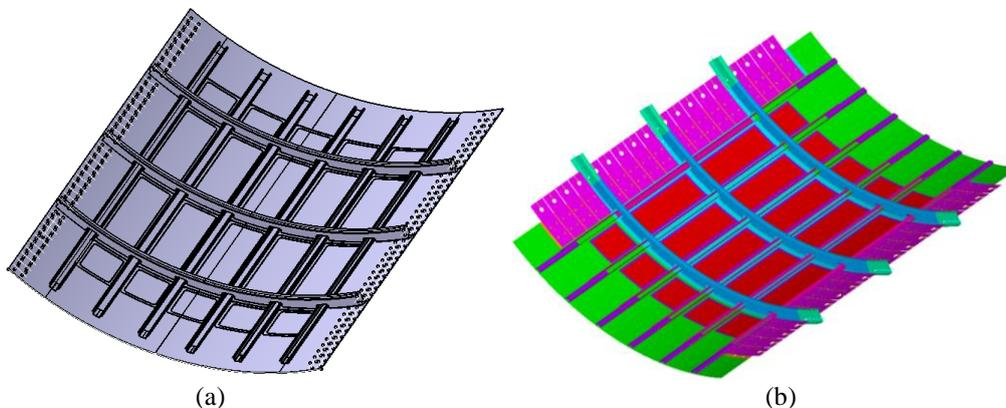
Figure 8: CAD drawing of 2nd modified panel design, provided by HAI (a), FE model in ANSYS APDL (b)
