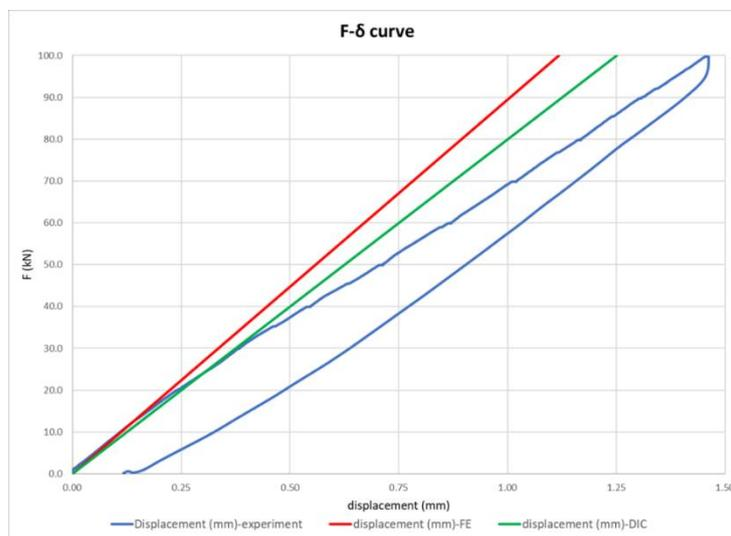
**Figure 2: Force-displacement curves of experiment (LVDT), DIC and FE**
