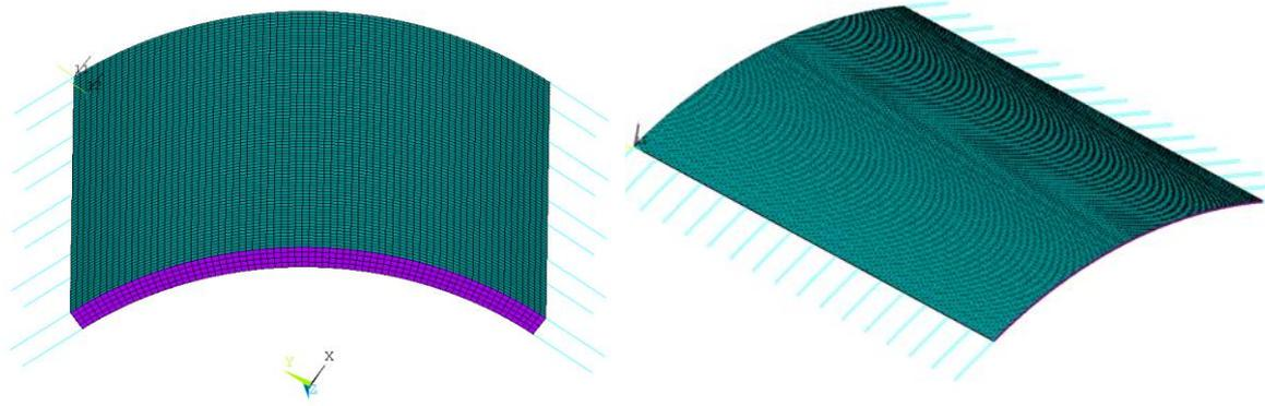
Figure 5: Arrangement of rods representing the omitted barrel segment (concept 2)
