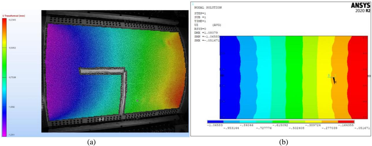
**Figure 11: Axial displacement contours, DIC (a), FE (b)**
