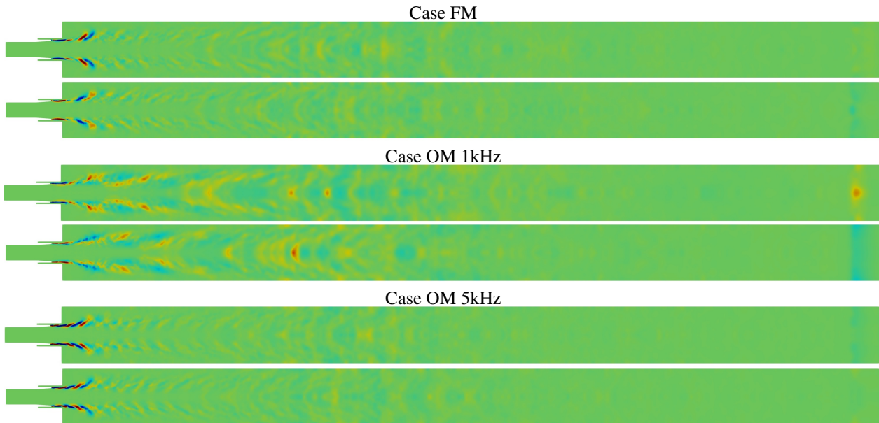
Figure 18: Longitudinal slices of phase-averaged heat release rate fluctuations (between -2 \cdot 10^{11} \text{W/m}^3 and 2 \cdot 10^{11} \text{W/m}^3 ) for \phi = 0 and \phi = \pi .
