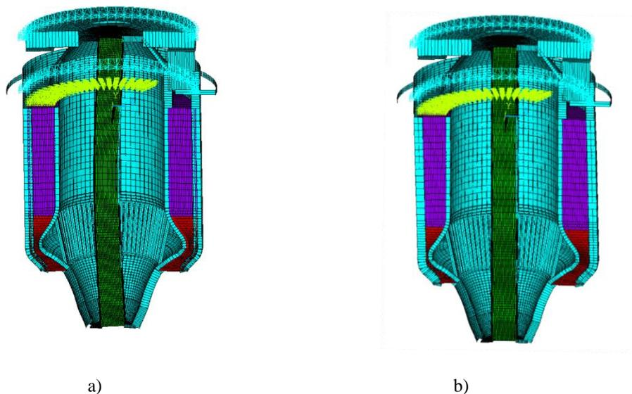
Figure 3: Natural transverse mode oscillation shapes of DemoP1: a) 673 Hz frequency mode, b) 1943 Hz frequency oscillation mode
