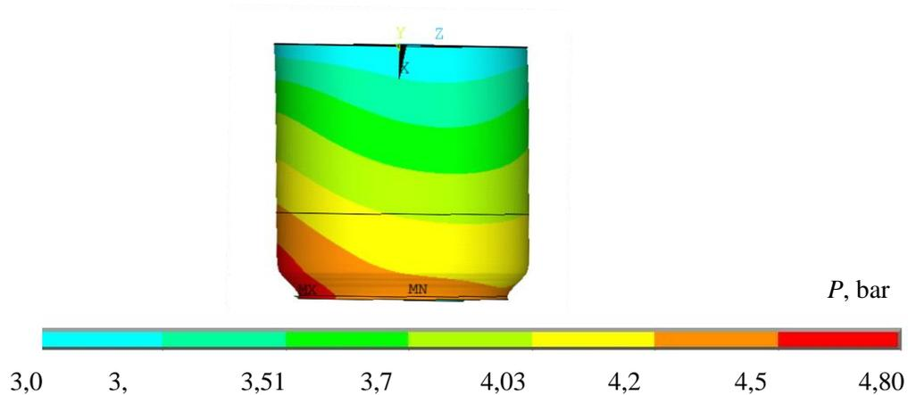
Figure 11: Distribution of gas pressure dynamic component in DemoP1 engine annular chamber at non-symmetric harmonic disturbance with 3 bar amplitude and transverse oscillations frequency of 2107 Hz after strengthening the pipeline and outer shell structure
