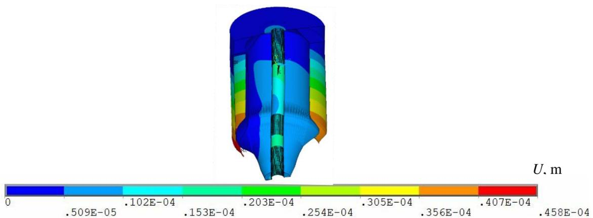
Figure 5: Distribution of dynamic (vibration) displacement components over the outer shell of the DemoP1 engine structure at non-symmetric harmonic disturbance with 3 bar amplitude and a transverse oscillation frequency of 834 Hz
