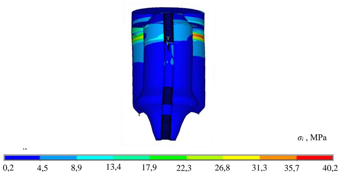
Figure 10: Dynamic stress components in the DemoP1 engine structure at non-symmetric harmonic disturbance with 3 bar pressure oscillation amplitude and transverse oscillations frequency of 2107 Hz after strengthening the pipeline and outer shell structure
