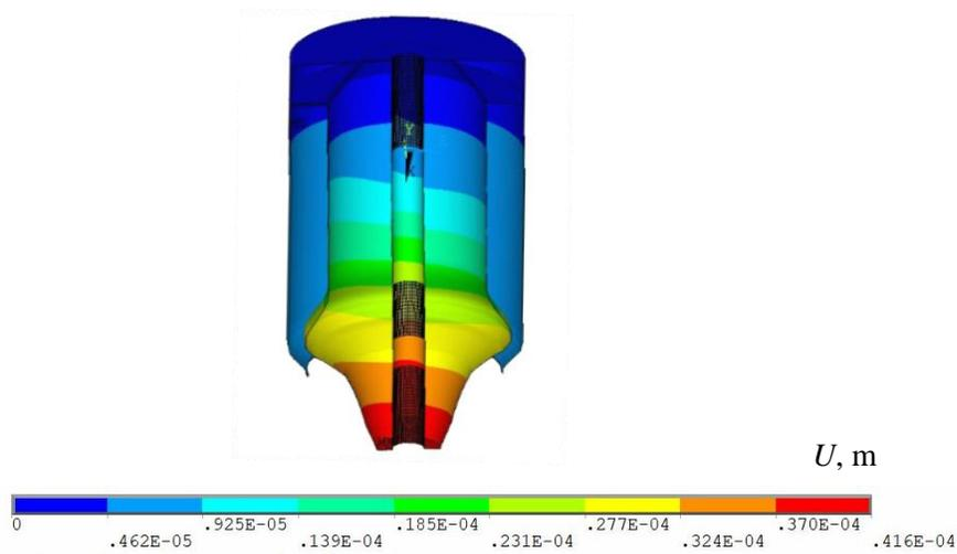
Figure 7: Dynamic displacement components in the DemoP1 engine structure for a non-symmetric harmonic disturbance with 3 bar amplitude and a transverse oscillations frequency of 1030 Hz after strengthening the pipeline and outer shell structure
