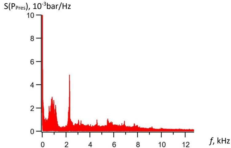
Figure 13: Spectral densities of  $S$  signals obtained after processing the oxidizer pressure oscillation sensor data  $P_{Pre}$  at the DemoP1 engine inlet within frequency range from 0 kHz to 12 kHz
