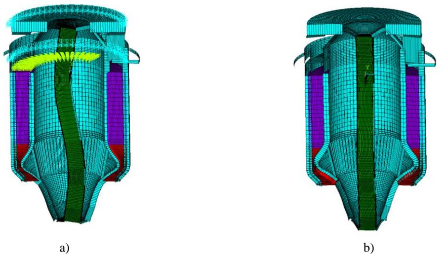
Figure 2: The natural longitudinal oscillation mode shapes of DemoP1: a) 2069 Hz frequency oscillation mode, b) 3212 Hz frequency oscillation mode
