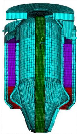
Figure 1: The graphic representation of the finite-element model of the DemoP1 engine annular combustion chamber (172272 elements)
