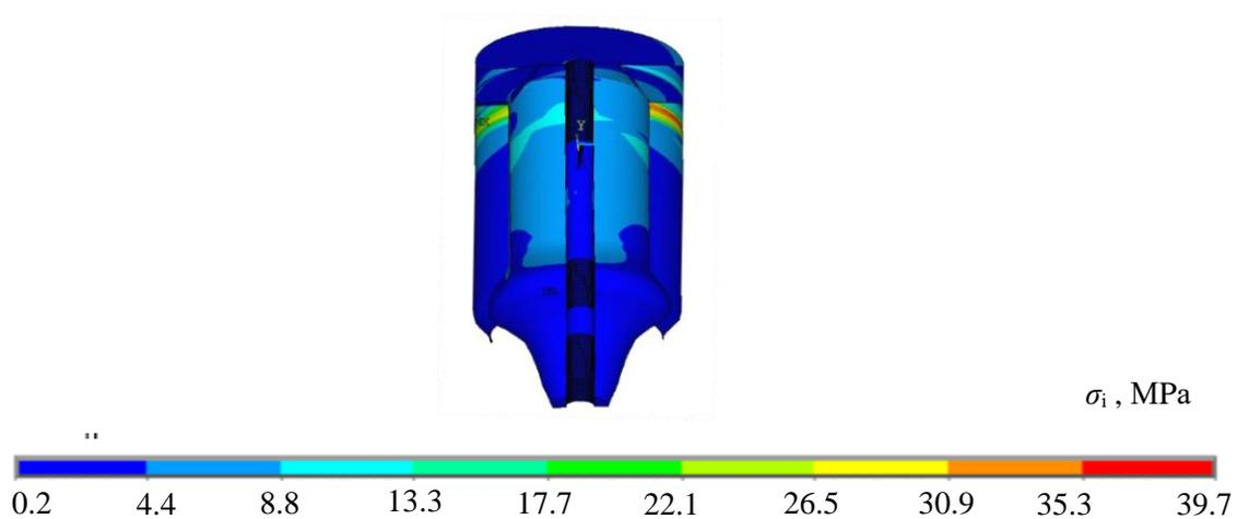
Figure 8: Dynamic stress components in the DemoP1 engine structure for a non-symmetric harmonic disturbance with 3 bar amplitude and a transverse oscillations frequency of 1030 Hz after strengthening the pipeline and outer shell structure ( $E=110$  GPa)
