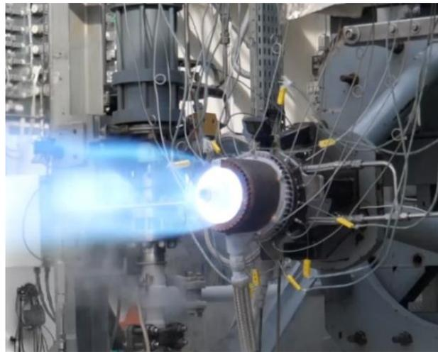
Figure 12: The LOX/LNG aerospike engine DemoP1 during a firing test
