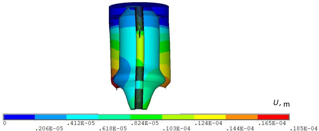
Figure 9: Dynamic displacement components in the DemoP1 engine structure at non-symmetric harmonic disturbance with 3 bar amplitude and transverse oscillations frequency of 2107 Hz after strengthening the pipeline and outer shell structure
