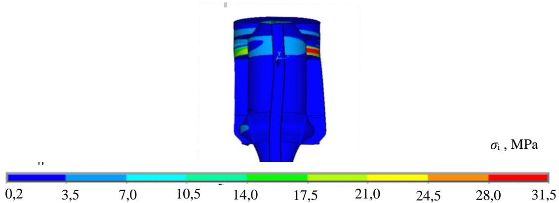
Figure 4: Dynamic stress components in the DemoP1 engine structure at non-symmetric harmonic disturbance with a 3 bar pressure amplitude and transverse oscillation frequency of 1834 Hz
