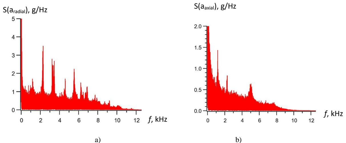
Figure 14: Spectral densities of  $S$  signals obtained after processing the transverse  $a_{radial}$  and axial  $a_{axial}$  accelerometer data from DemoP1 engine structure within frequency range from 0 kHz to 12 kHz
