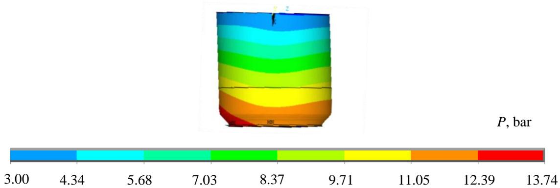
Figure 6: Distribution of gas pressure dynamic component in the annular chamber of DemoP1 for a non-symmetric harmonic disturbance with 3 bar amplitude and a transverse oscillations frequency of 1834 Hz
