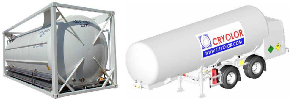
Figure 6: Standard ISO container for LNG transport (12,2m x 2,4m x 2,6m ~18 tons of LNG) versus Cryolor tank
