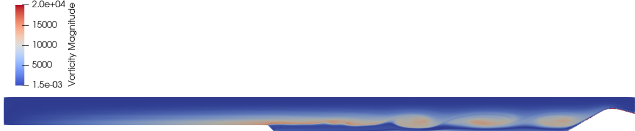
Figure 9: Vortex shedding phenomena appearance in the chamber
