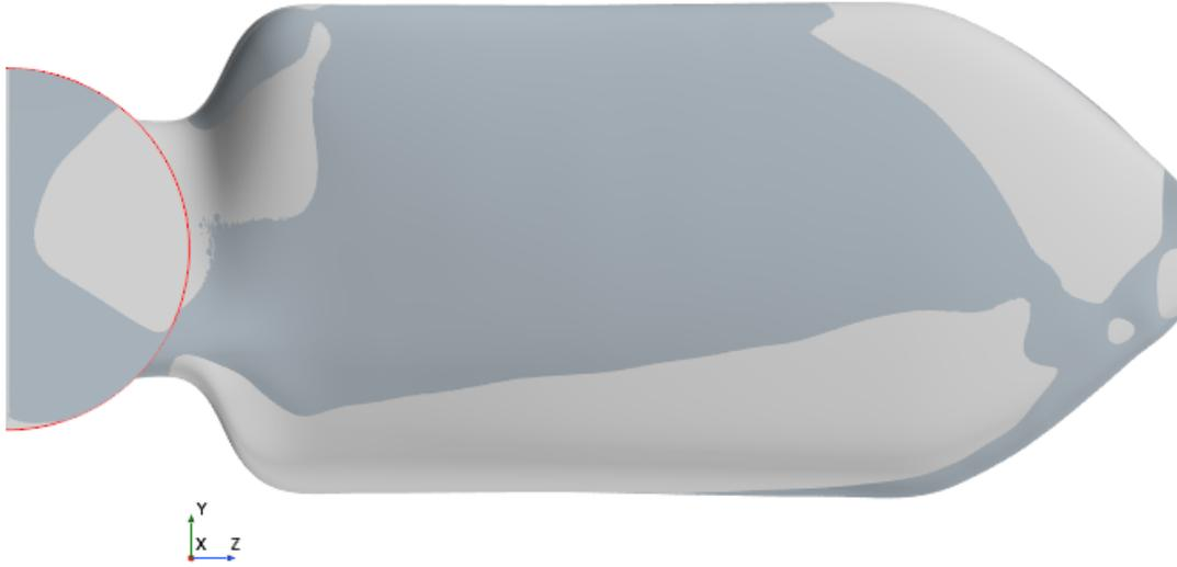
Figure 9: Comparison between original(Light grey) and morphed surface(Dark Grey) after the final adjoint iteration.
