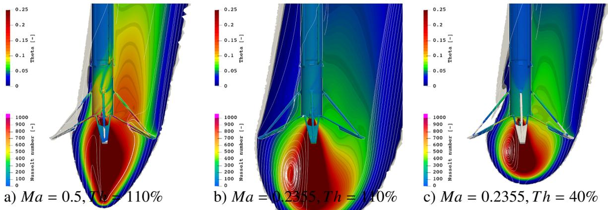
Figure 8: Influence of Mach number and thrust level. Slices through the centre line with velocity stream lines, dimensionless temperature  $\Theta$  slice and dimensionless heat flux  $Nu$  on the vehicle surface for  $AoA = 170^\circ$  and for a)  $Ma = 0.5, Th = 110\%$ , b)  $Ma = 0.2355, Th = 110\%$  and c)  $Ma = 0.2355, Th = 40\%$ .
