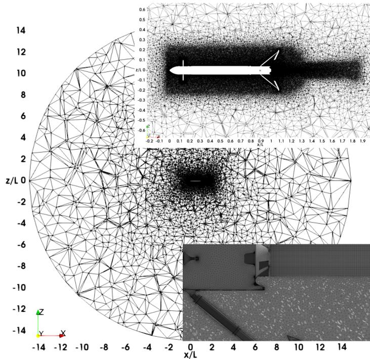
Figure 1: Computational grid for CALIC UVO configuration with zoomed regions for local refinement and block structured region.
