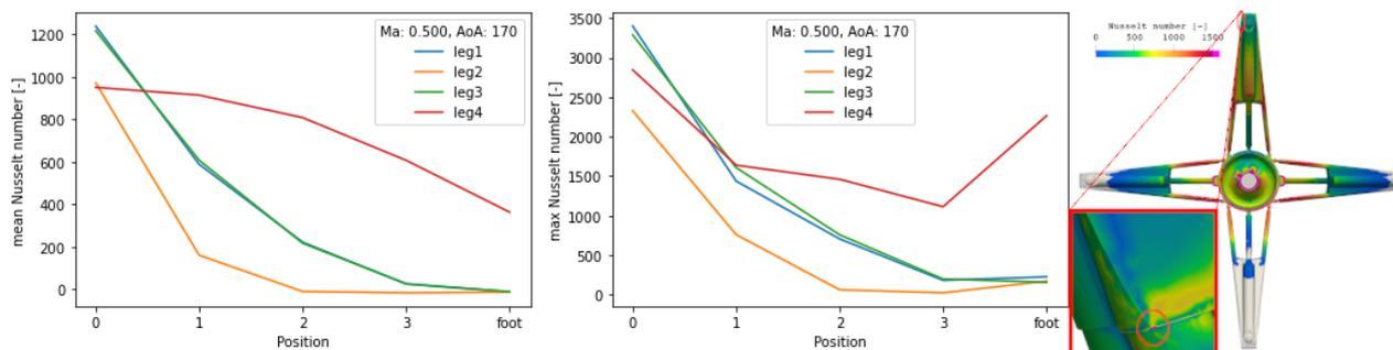
Figure 4: Plots of mean and max dimensionless heat flux  $Nu$  for different sections of the landing legs for  $Ma = 0.5$ ,  $\rho = 1.18\text{kg m}^{-3}$  and  $AoA = 170^\circ$ . On the right the bottom view of the landing legs with  $Nu$  contouring and a cut out showing the heat flux peak.
