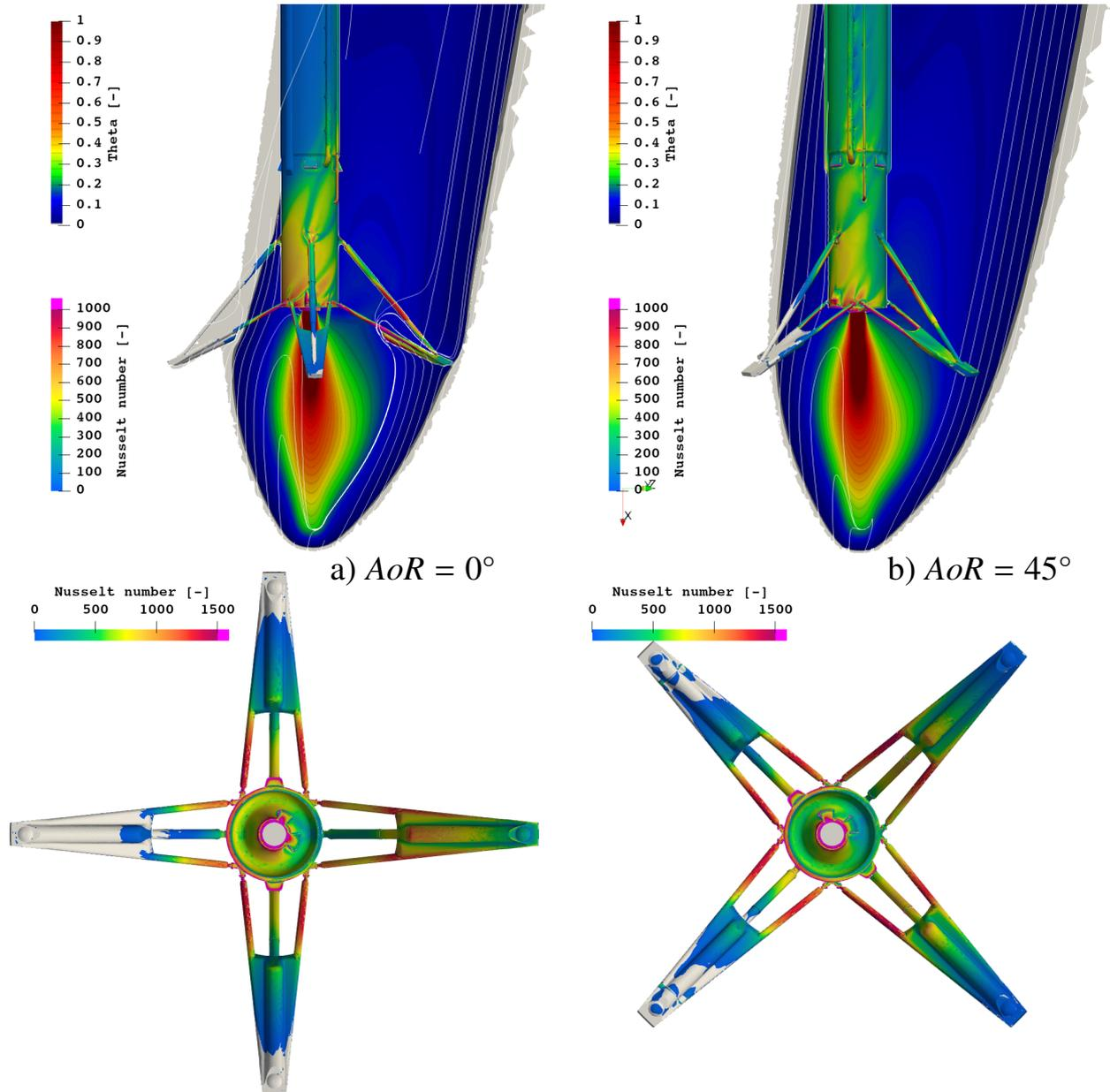
Figure 7: Influence of angle of roll. On the left a)  $AoR = 0^\circ$ , on the right b)  $AoR = 45^\circ$ . Top row showing slices through the centre line with velocity stream lines, dimensionless temperature  $\Theta$  slice and dimensionless heat flux  $Nu$  on the vehicle surface for  $Ma = 0.5$  and  $AoA = 170^\circ$ . Bottom row showing bottom view of landing legs with  $Nu$ .
