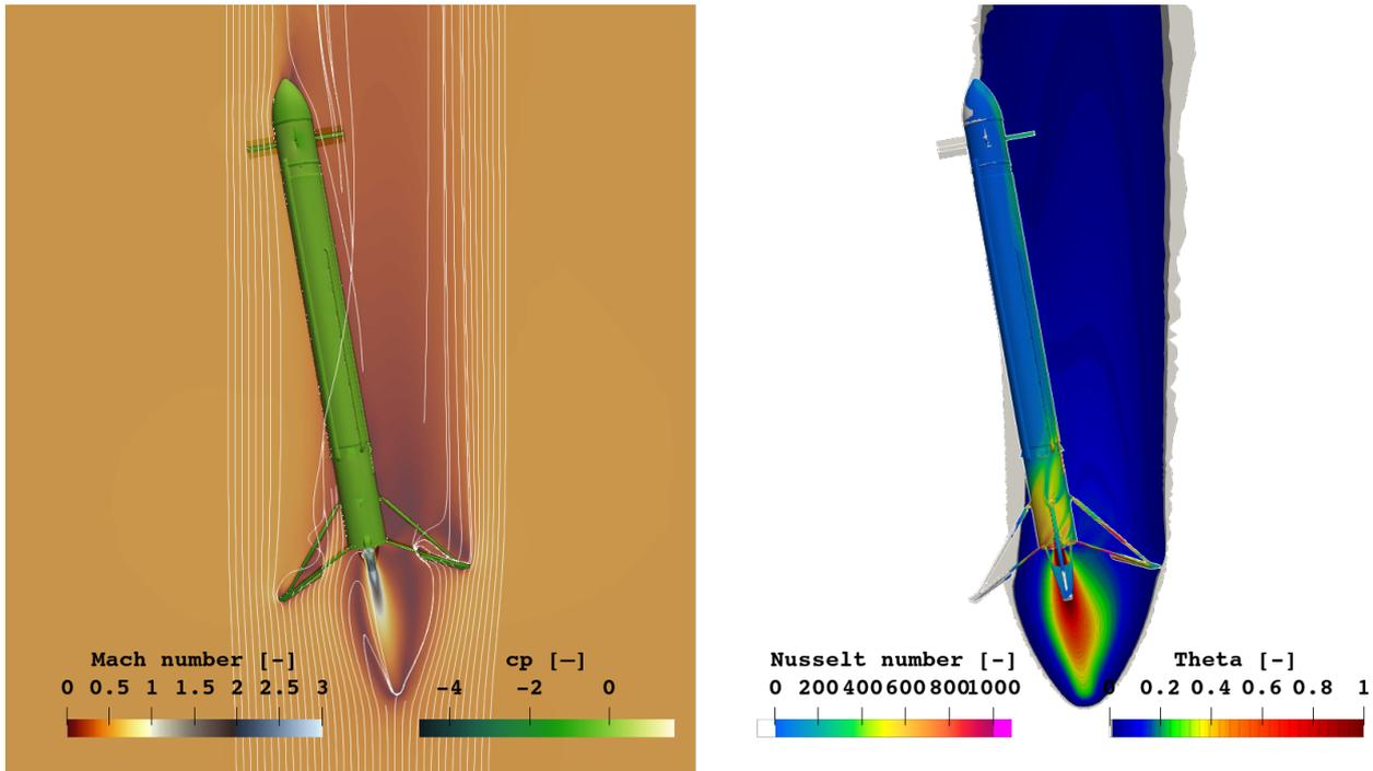
Figure 3: Flow field of Callisto UVO configuration at  $Ma = 0.5$ ,  $\rho = 1.18\text{kg m}^{-3}$  and  $AoA = 170^\circ$ . On the left, Mach number  $Ma$  slice through the centre line with velocity stream lines and  $c_p$  on the vehicle surface. On the right, dimensionless temperature  $\Theta$  slice and dimensionless heat flux  $Nu$  on the vehicle surface.
