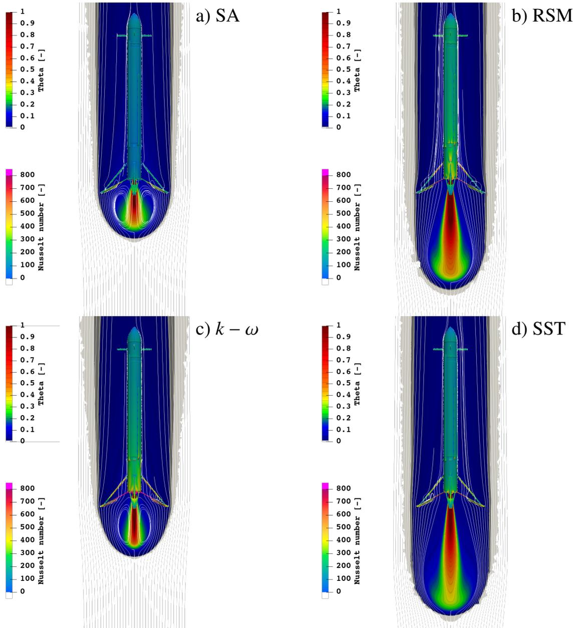
Figure 9: Comparison of four different turbulence models. Side view of a centre line slice cut of dimensionless temperature  $\Theta$  and dimensionless heat flux  $Nu$  on the vehicle surface.  $Ma = 0.299$ ,  $\rho = 1.127\text{kg m}^{-3}$  and  $AoA = 180^\circ$ .
