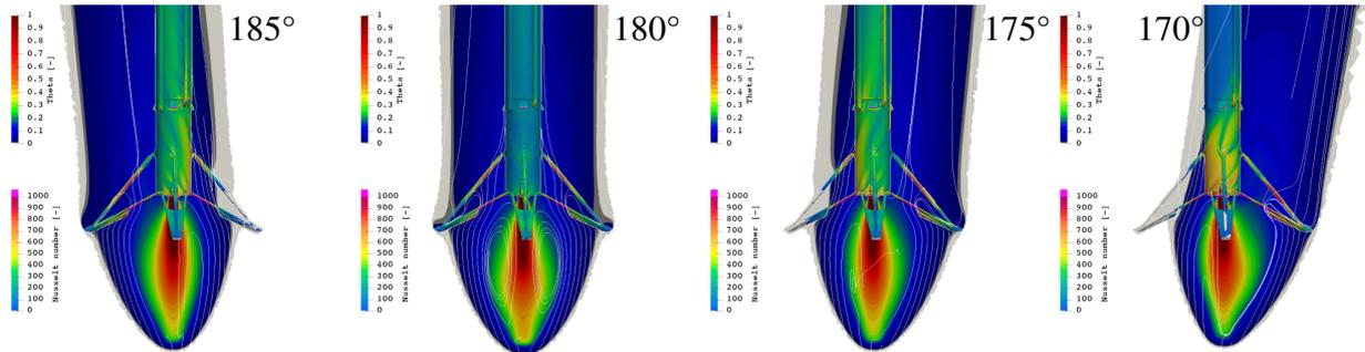
Figure 5: Influence of angle of attack. Slices through the centre line with velocity stream lines, dimensionless temperature  $\Theta$  slice and dimensionless heat flux  $Nu$  on the vehicle surface for angles of attack  $AoA = 185^\circ, 180^\circ, 175^\circ$  and  $170^\circ$ .
