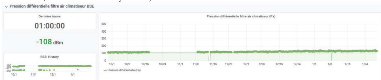
Figure 6 : Dashboard of BSE air conditioner differential pressure measurements
