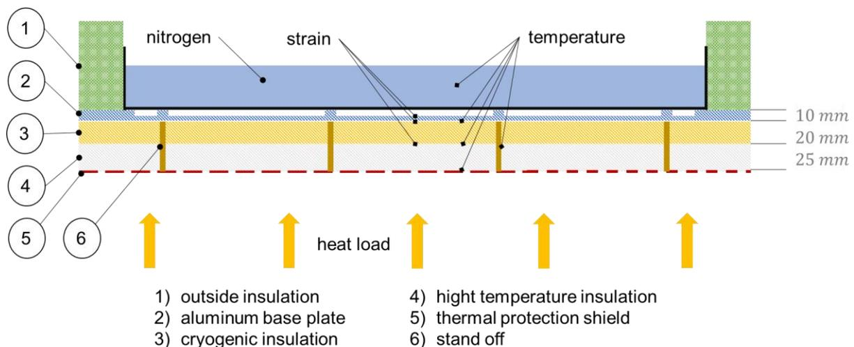
Figure 7: Sketch of cross section of the ITO representing metallic tank structures
