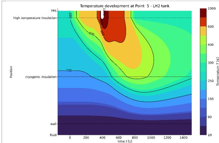
Figure 1: Exemplary evolution of temperature over time for an architecture without purge gap consisting of an external cryogenic insulation (PU-foam, 20mm) and a high temperature insulation (altramat, 25mm) and an external panel (CMC, 3mm)
