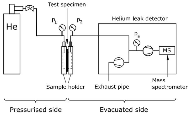
Figure 10: Scheme of the permeation test rig.
