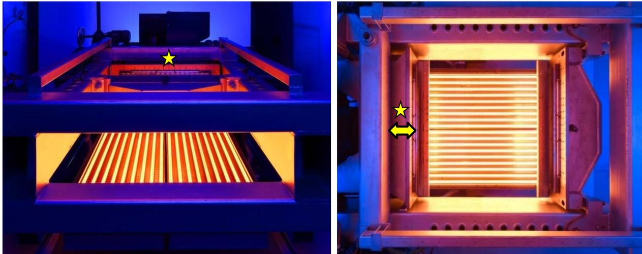
Figure 11: Front view (left) and top view (right) of the THERMEX facility. The structure is placed above the infrared heating unit. The star denotes the clamped side of the structure that applies axial forces.
