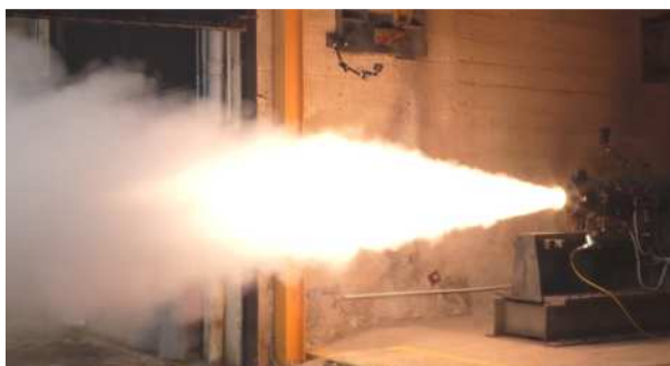
Figure 13 : NMF HTPB/AP/Al grain firing
