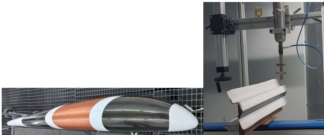
Figure 13: Demonstrators. On the left, HPCS of Cu onto a full-sized real aircraft wing salmon made of thermoset (epoxy) based CFRP, with PPF. On the right, LPCS of a PEEK-Al mixture onto an “omega-shaped” part made of thermoplastic CFRP.
