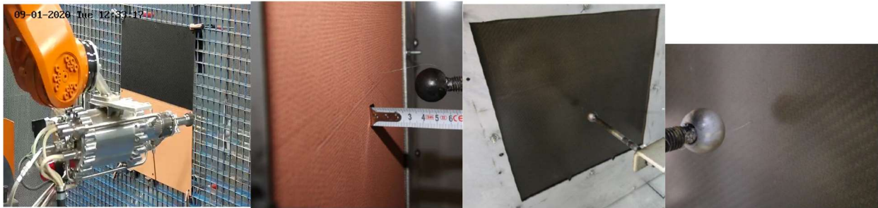
Figure 11: From left to right: HPCS pure copper coating on CFRP+PPF(50 \mu m), reference mesh before test.
