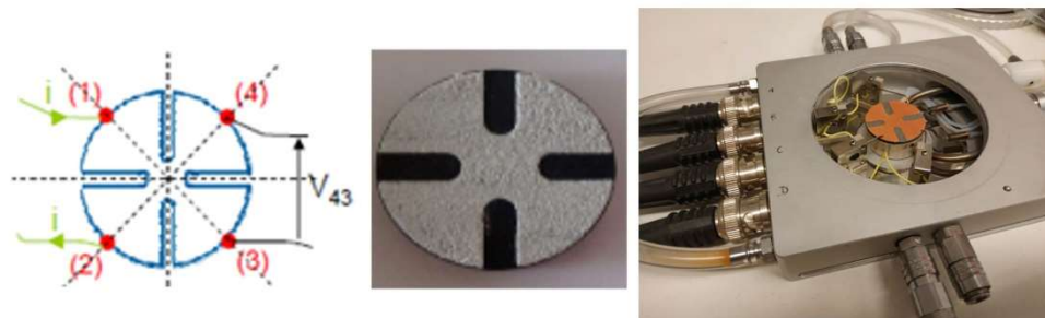
Figure 2: on the left, schematic view of the Van der Pauw method; at the center, picture of one of the tested samples; on the right, picture of the measuring set up.
