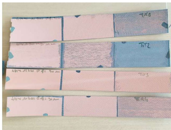
Figure 4: HPCS copper coatings obtained with different spraying conditions. Substrates, made of thermoset CFRC, had, in each column, the same PEEK PPF thickness (300 \mu\text{m} on the left, 50 \mu\text{m} on the middle and 25 \mu\text{m} on the right).
