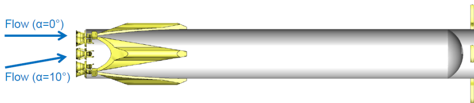
Figure 2: Flow direction with respect to the vehicle for the two angles of attack \alpha = 0^\circ and \alpha = 10^\circ .
