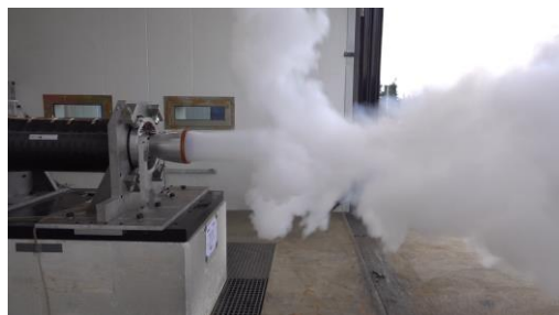
Figure 4. Hot firing test of the new hybrid motor design. Time 0.1 sec. - Monopropellant phase.
