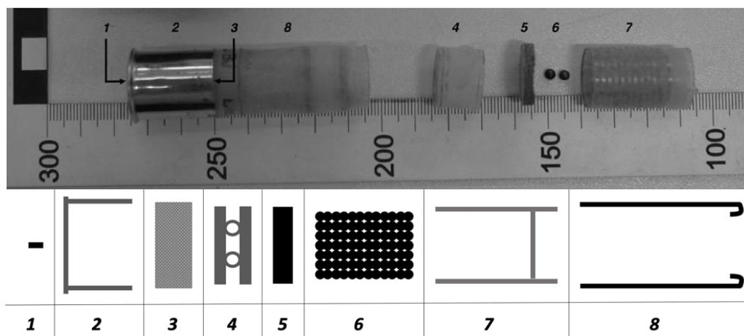
Figure 3: Exploded view of the ammunition [25]
