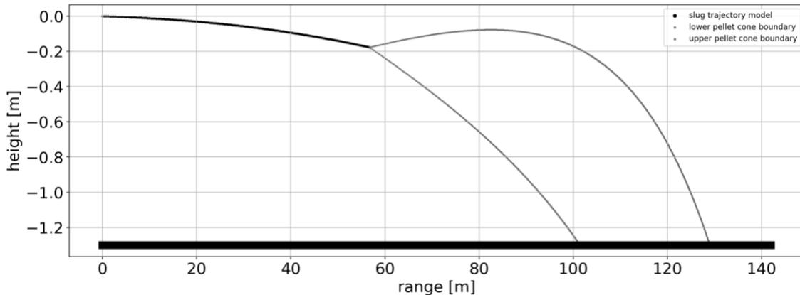
Figure 10: Result of the PMM with a barrel elevation of  $-0.05^\circ$  and a muzzle velocity of 396.48 m/s [32].
