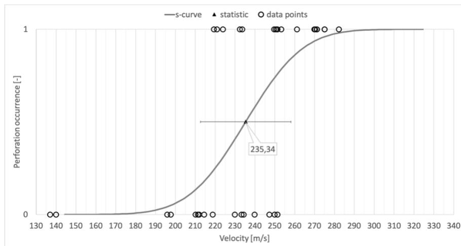
Figure 11: Results of the determination of the ballistic limit  $v_{50}$  of the UAV shell
