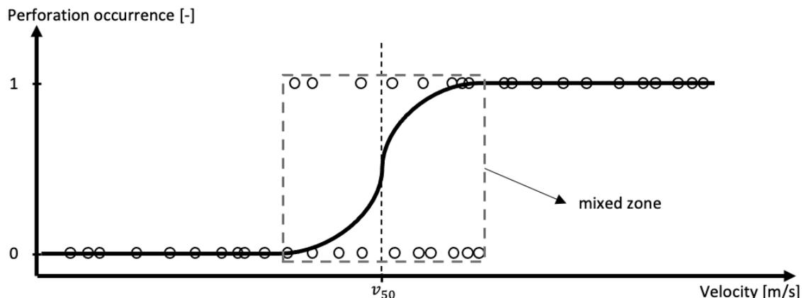
Figure 9: Typical shape of the result after processing experiment data with Probit Analysis.
