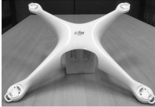
Figure 5: DJI Phantom upper shell used for determination of the ballistic limit
