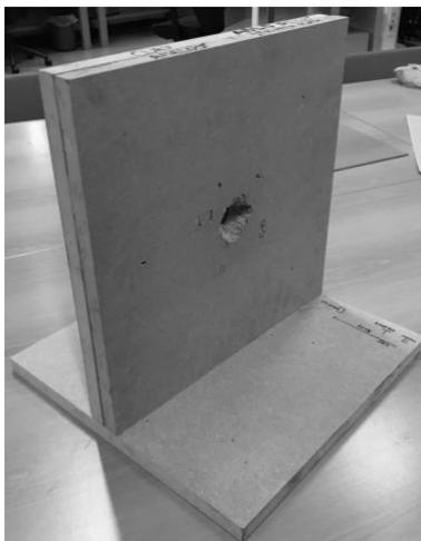
Figure 7: The stripper plate that is used to capture the sabots and that allows the pellet to pass through the hole.
