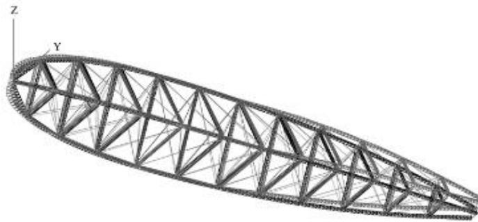
Figure 19: Finite Element Model design for a primary structure (semi-rigid airship concept)
