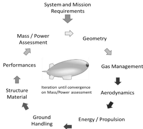
Figure 1: Overall Design Loop
