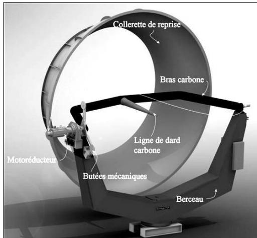
Figure 12: CAD of PQR rig
