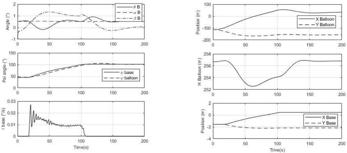
Figure 5: Tethered balloon trajectory characteristics in a wind heading change
