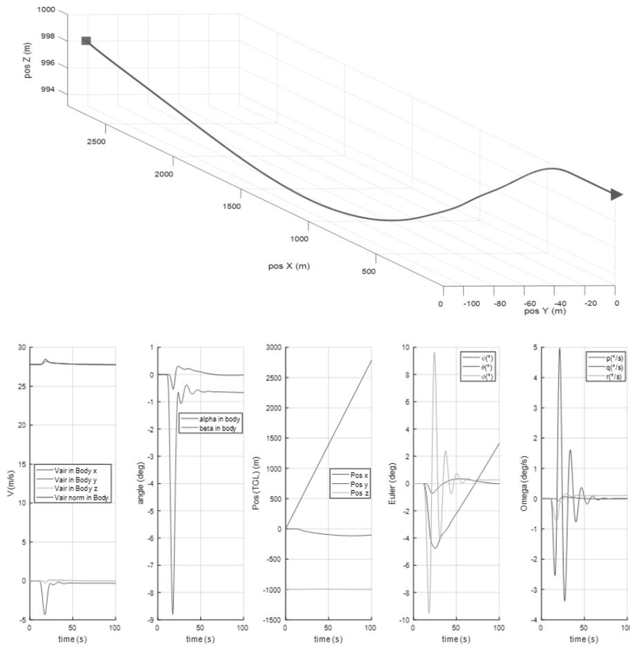
Figure 10: Effect of a lateral (1+cos) shape gust on a trimmed level flight (large transport airship).
