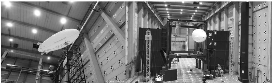
Figure 18: free flight laboratory B20 at ONERA and flight of a 5m model through the lateral wind generator.
