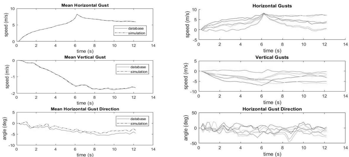
Figure 21: Results obtained from gust model ( $L/2 = 150\text{m}$ ,  $V_{\text{gust}} 7.6\text{m/s}$ ,  $V_{\text{airship}} 100\text{km/h}$ )
