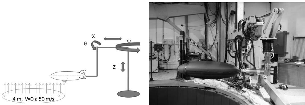
Figure 15: Tests on ellipsoid in the vertical wind tunnel SV4 at ONERA-Lille – effects of transverse flow
