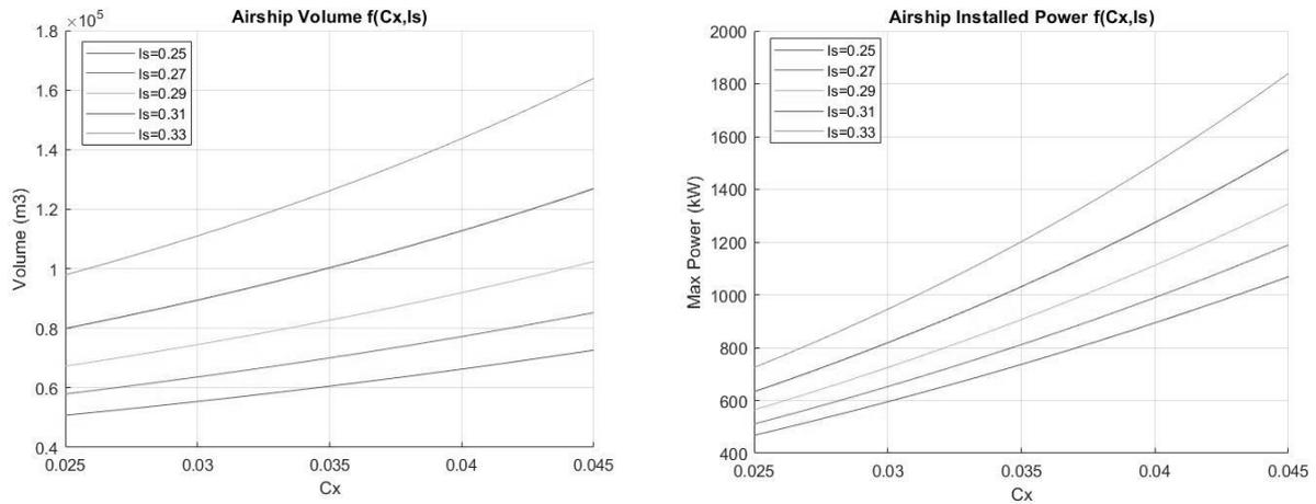
Figure 2: Volume and Installed power
