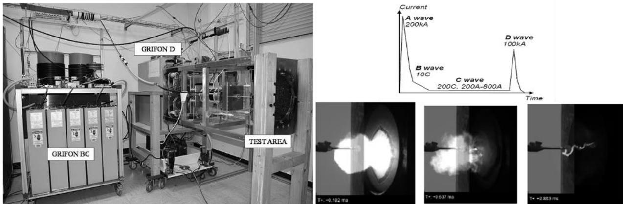
Figure 20 : Views of GRIFON Lightning strike test facility. Typical waves for Lightning strikes
