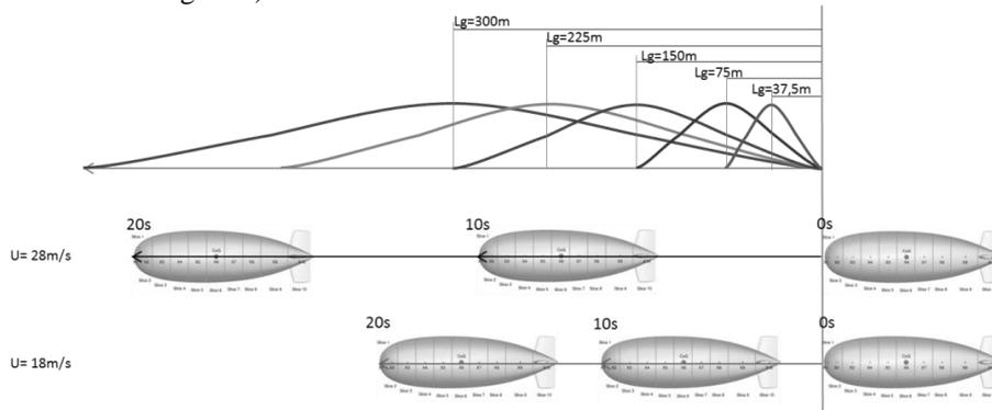
Figure 9: representation of gust relative to regulation- application to a 150m long airship
