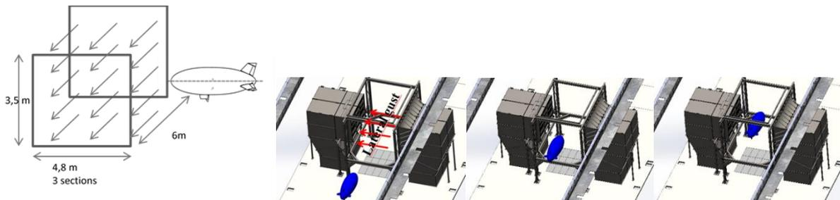
Figure 17: Schema of the lateral wind generator and flight of a 5m model
