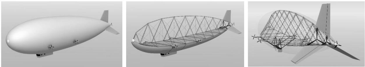
Figure 3: Visuals from a concept of medium altitude long endurance surveillance airship
