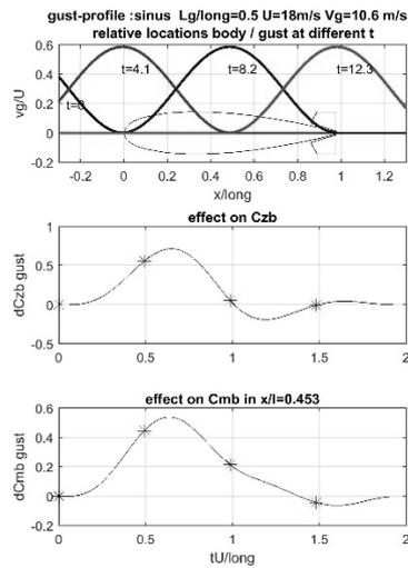
Figure 16: Simulation of flight through a  $(1+\cos)$  vertical gust – induced normal force and pitching moment
