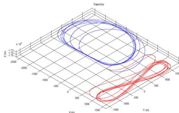
Figure 8: Station keeping trajectory for a stratospheric airship
