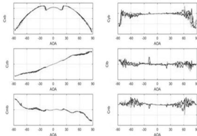
Figure 14: Sample of aerodynamic coefficients (body frame) obtained from windtunnel tests
