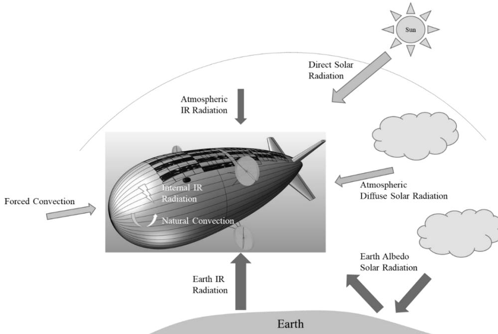
Figure 7: Thermal environment for an airship
