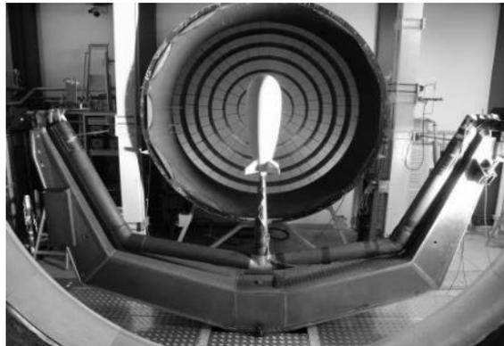
Figure 13: Stratobus™ mockup tested in L1 windtunnel facility (Mockup is 1m length)
