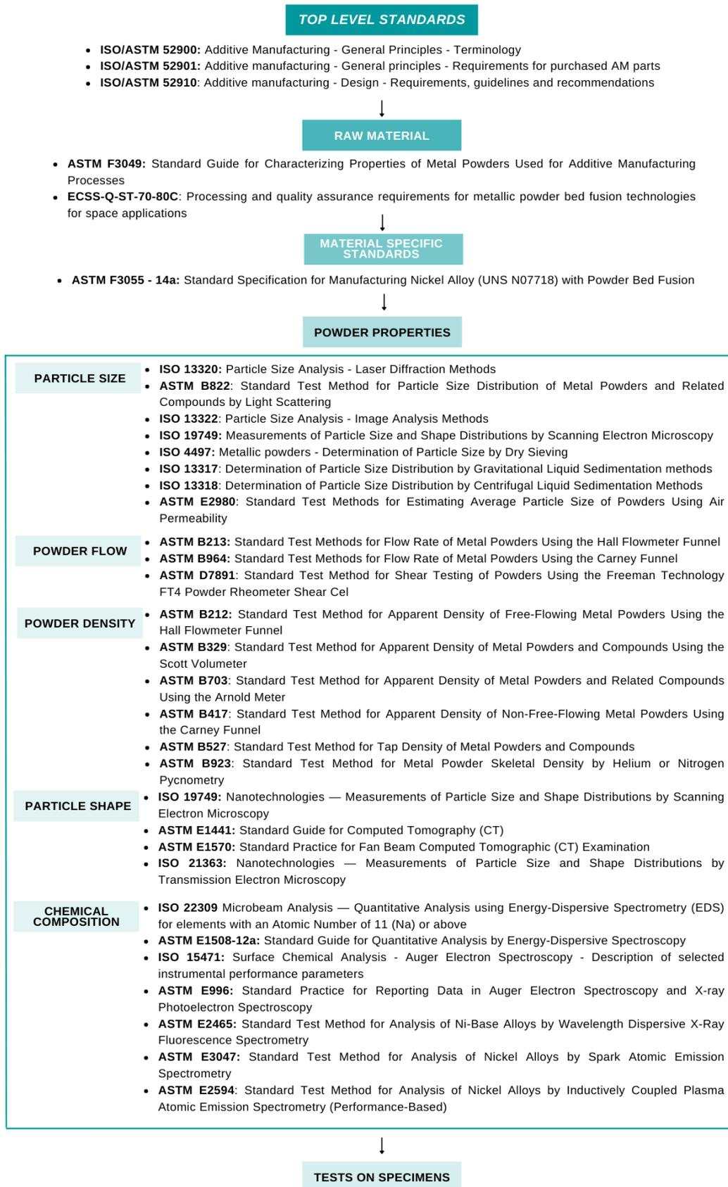
Figure 3: Standard identification process tailored for IN718 powders.
