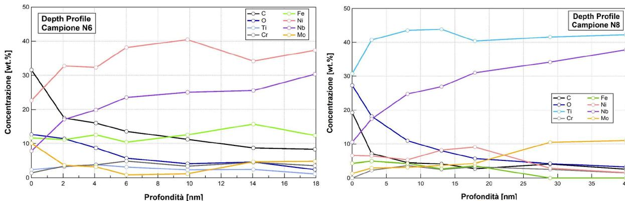
Figure 12: AES profile of sample N6 (on the left) and N8 (on the right).
