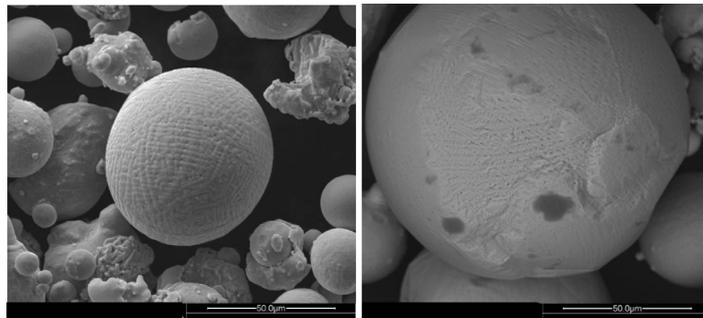
Figure 4: SEM images reporting particle surface roughness (on the left) and particle surface contamination (on the right).
