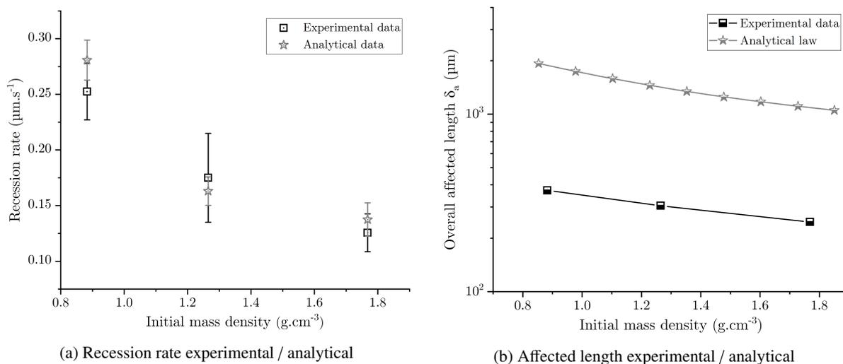
Figure 6: Comparison of analytical recession rate and affected length values to experimental data
