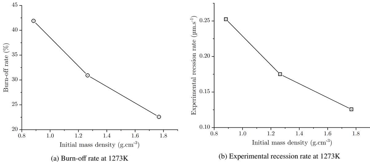
Figure 3: Experimental results of burn-off and recession rates after half an hour of oxidation at 1273K
