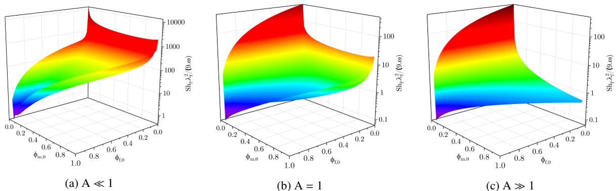
Figure 8: Operating graphs of the affected length  $\delta_a$  with environmental conditions depending on fibers behavior ( $Sh_f$ ) and architectural parameters ( $\phi_{f,0}, \phi_{m,0}$ )
