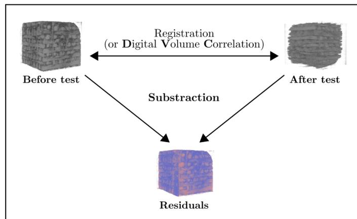
Figure 1: Schematic of the Digital Volume Correlation method
