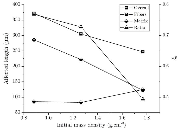
Figure 4: Characterization results of affected lengths after oxidation after half an hour of oxidation at 1273K
