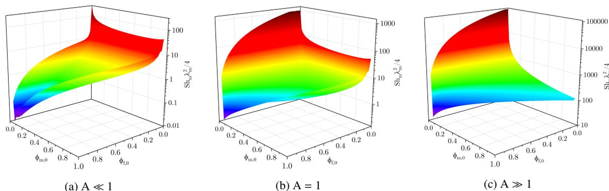
Figure 9: Operating graphs of the affected length  $\delta_a$  with environmental conditions depending on matrix behavior ( $Sh_m$ ) and architectural parameters ( $\phi_{f,0}$ ,  $\phi_{m,0}$ )
