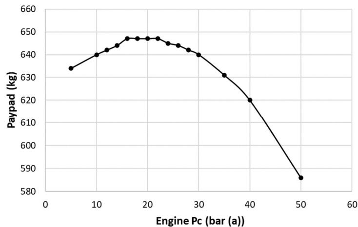
Figure 6 Variation in payload with change in engine chamber pressure.
