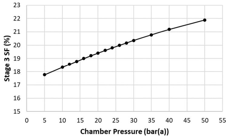
Figure 5 Variation in stage-3 SF with change in engine chamber pressure.
