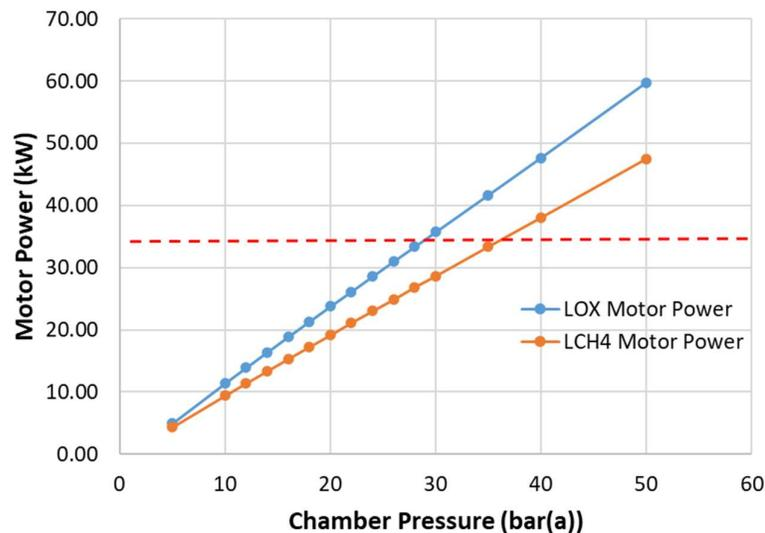
Figure 4 Variation in pump power with change in engine chamber pressure.
