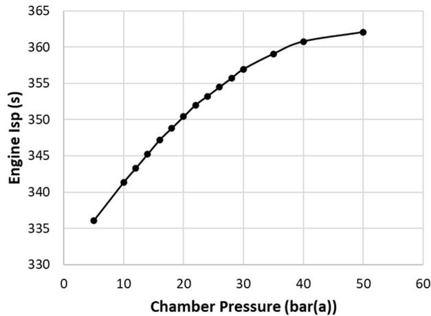
Figure 3 Variation in engine Isp with change in engine chamber pressure.
