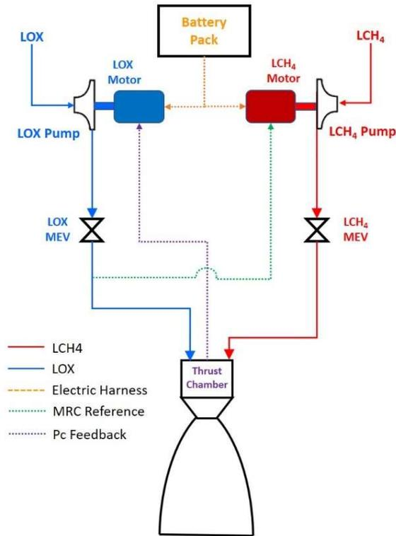
Figure 1 EPFC engine flow schematic
