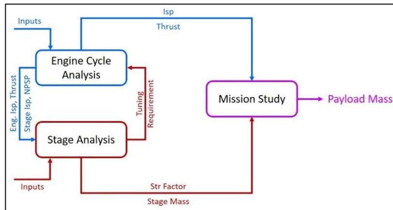
Figure 2 Architecture of integrated stage cycle analysis toolkit.
