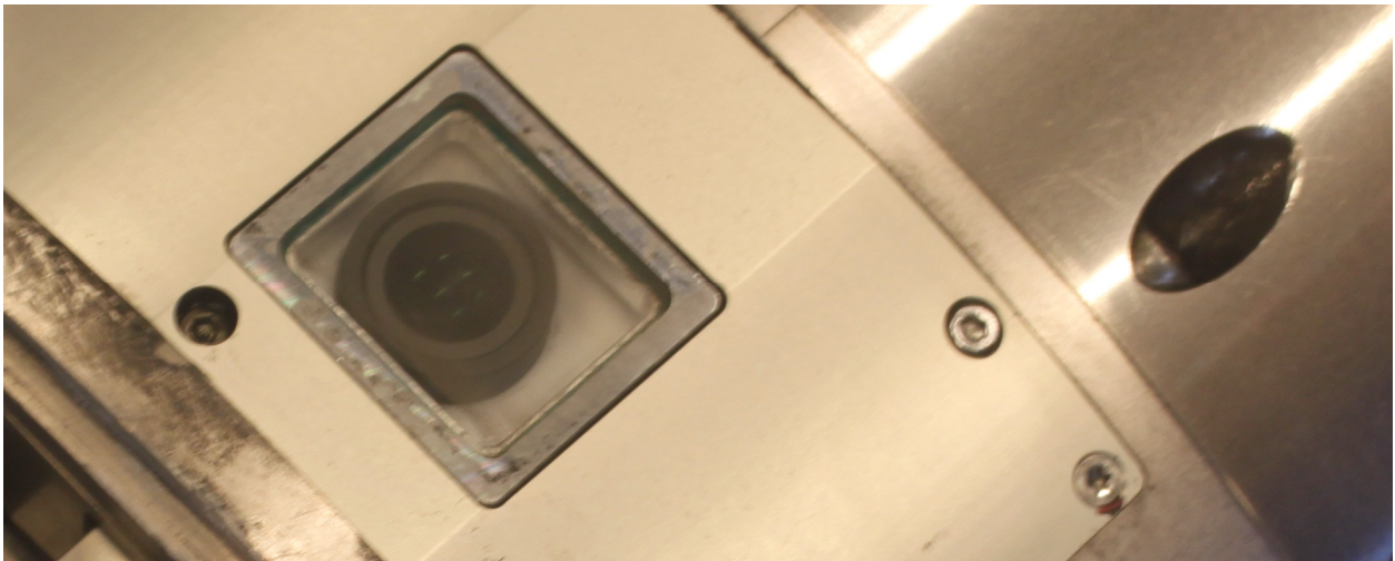
Figure 2: Side-looking GoPro HERO3+ camera. The lens was protected by a thin pane of glass
