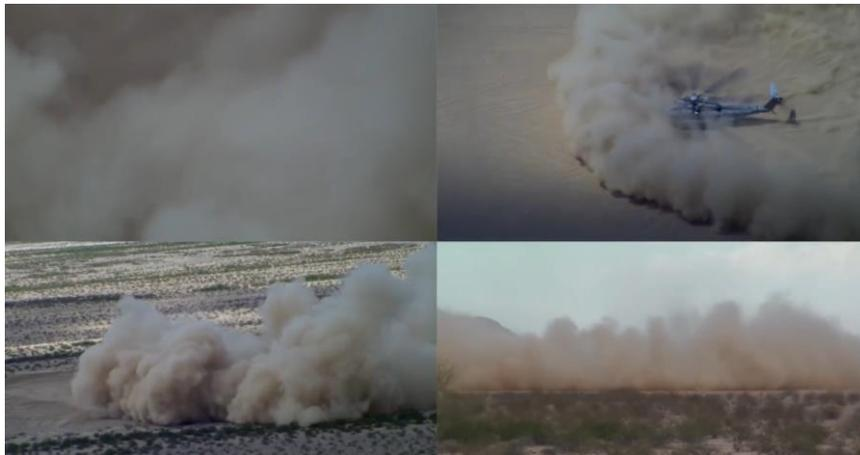
Figure 1: CH-53 helicopter in brownout condition. [1]
