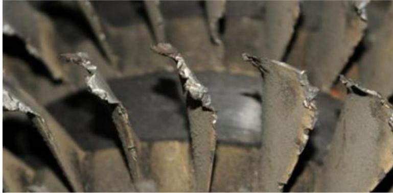
Figure 2: Damaged compressor blades. [3]
