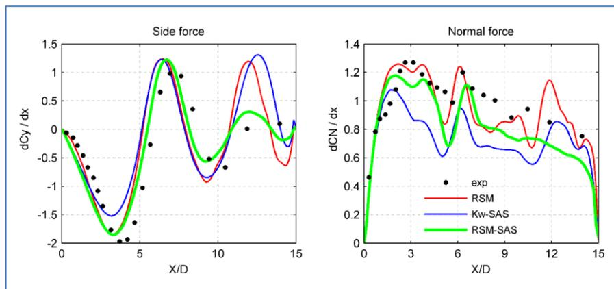
Figure 8: Averaged local side and normal force coefficients at Mach number  $Ma = 0.2$ , Reynolds number  $Re = 2 \cdot 10^6$  and angle of attack  $\alpha = 45$  degrees within a period of  $T = 0.1$  s. Structured mesh.  $\omega$ -based *RSM-SAS* model.
