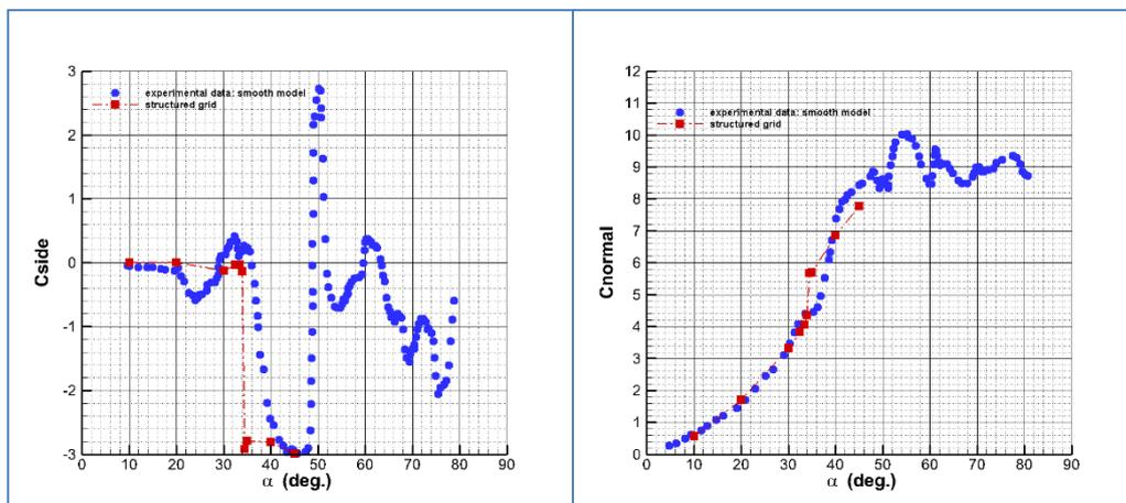
Figure 11: Left: Side force coefficient versus angle of attack. Right: Normal force coefficient versus angle of attack.  $Ma = 0.2$ ,  $Re = 2 \cdot 10^6$ . Structured grid solutions (red squares) compared to experimental data (in blue dots) for the smooth model (extracted from reference [11]).
