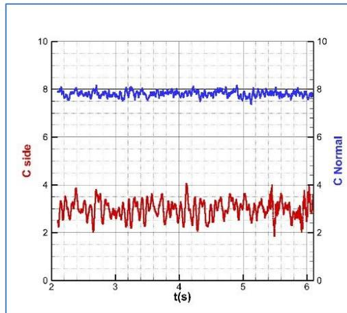
Figure 6: Time history for the side and normal force coefficients at Mach number  $Ma = 0.2$ , Reynolds number  $Re = 2 \cdot 10^6$  and angle of attack  $\alpha = 45$  degrees within a time of  $T = 4$  s. Structured mesh.  $\omega$ -based RSM-SAS model.
