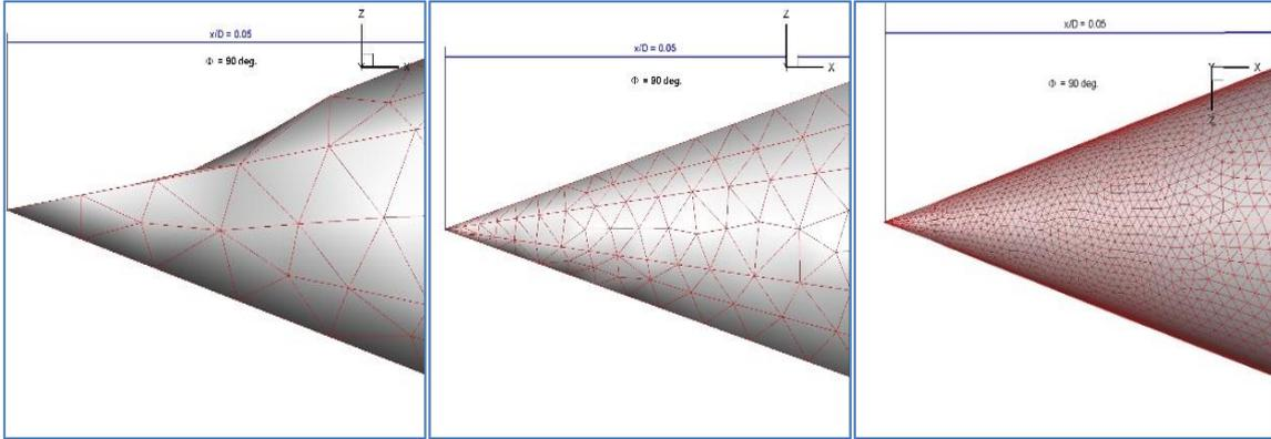
Figure 3: Detail of the unstructured grid at  $x/D < 0.05$ . Left: mesh generated with  $m = 3$ . Center: Mesh generated with  $m = 8$ . Right: finer mesh generated with  $m = 8$ .
