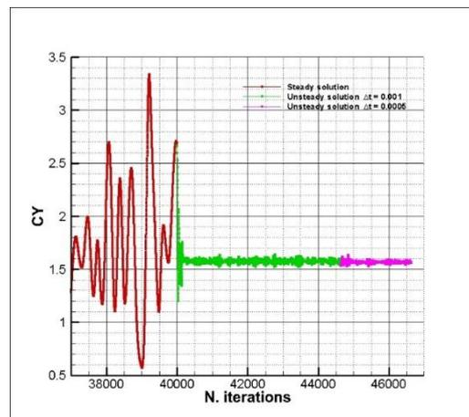
Figure 5: Side force coefficient versus number of iterations at Mach number  $Ma = 0.2$ , Reynolds number  $Re = 2 \cdot 10^6$  and angle of attack  $\alpha = 45$  degrees: Steady and transient calculations for two time steps. Structured grid.
