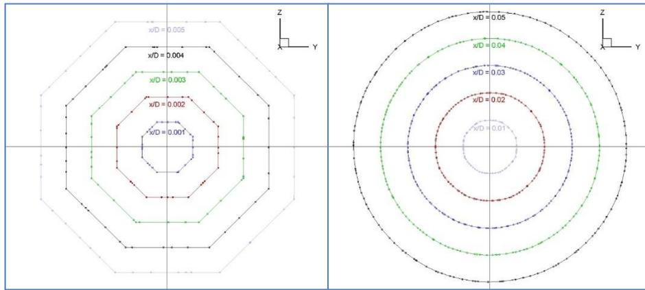
Figure 4: Left: Surface mesh cross sections at  $x/D = 0.001$  to  $x/D = 0.005$ . Right: Surface mesh cross sections at  $x/D = 0.01$  to  $x/D = 0.05$ . Unstructured grid.
