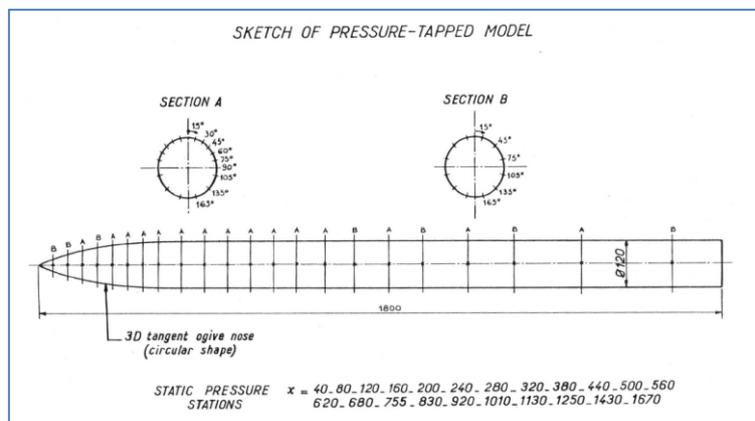
Figure 1: Sketch of the GARTEUR AG04 missile geometry and pressure taps (reprinted from [10]).
