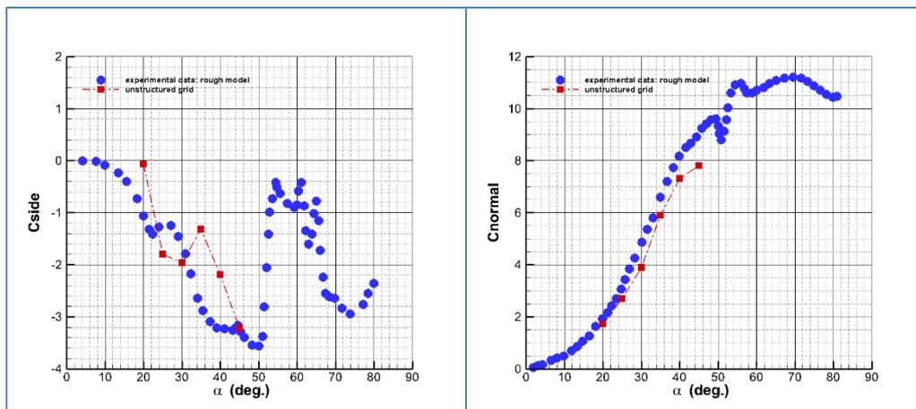
Figure 12: Left: Side force coefficient versus angle of attack. Right: Normal force coefficient versus angle of attack.  $Ma = 0.2$ ,  $Re = 2 \cdot 10^6$ . Unstructured grid solutions (red squares) compared to experimental data (in blue dots) for the rough model (extracted from reference [11]).
