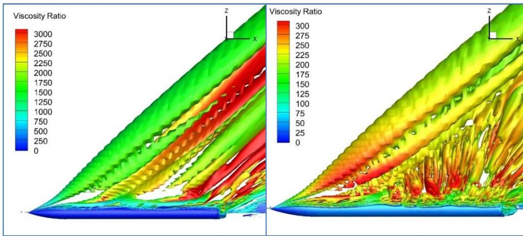
Figure 9: Iso surface of positive  $Q$  function (up to 5000) colored with turbulent viscosity ratio at Mach number  $Ma = 0.2$ , Reynolds number  $Re = 2 \cdot 10^6$  and angle of attack  $\alpha = 45$  degrees. Left: *k- $\omega$  SST-SAS* model. Right:  $\omega$ -based *RSM-SAS* model. Structured grid.
