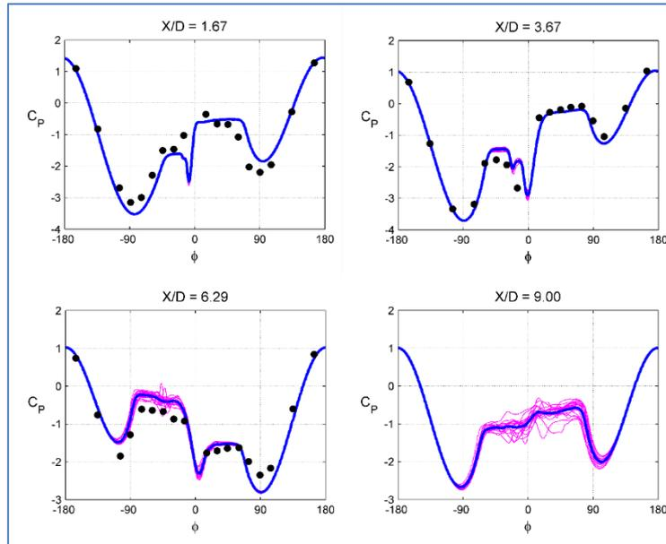
Figure 10: Pressure coefficients in circumferential direction at Mach number  $Ma = 0.2$ , Reynolds number  $Re = 2 \cdot 10^6$  and angle of attack  $\alpha = 45$  degrees within a period of  $T = 0.1$  s at four sections. Structured mesh.  $\omega$ -based RSM-SAS model solutions and experimental data (black dots).
