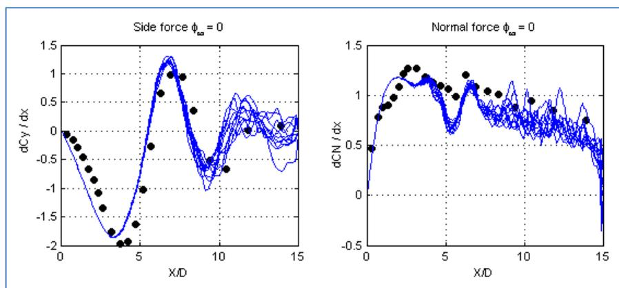
Figure 7: Several local side and normal force coefficients at Mach number  $Ma = 0.2$ , Reynolds number  $Re = 2 \cdot 10^6$  and angle of attack  $\alpha = 45$  degrees taken within a period of  $T = 0.1$  s in intervals of  $\Delta t = 0.005$  s. Structured mesh.  $\omega$ -based RSM-SAS model solutions and experimental data (black dots).
