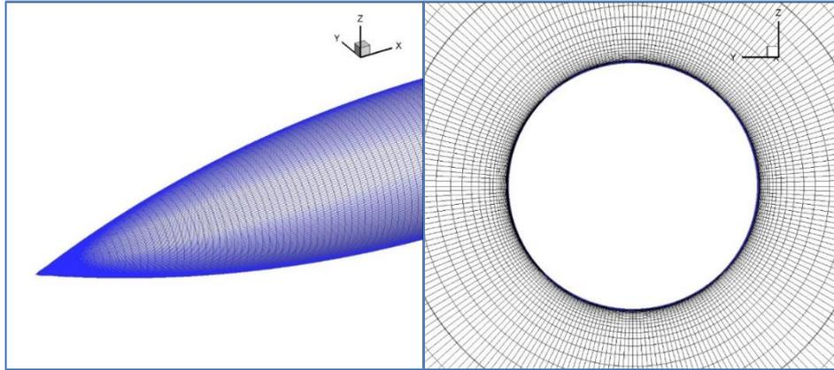
Figure 2: Detail of the structured grid: Left: Surface mesh on the nose. Right: Transversal plane y-z.
