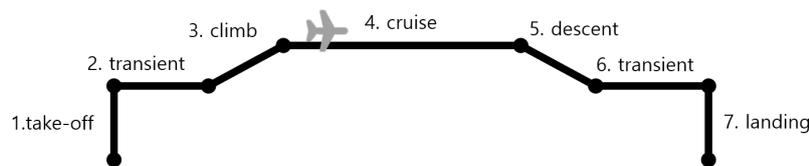
Figure 2: Profile for tiltrotor and lift-cruise type UAM
