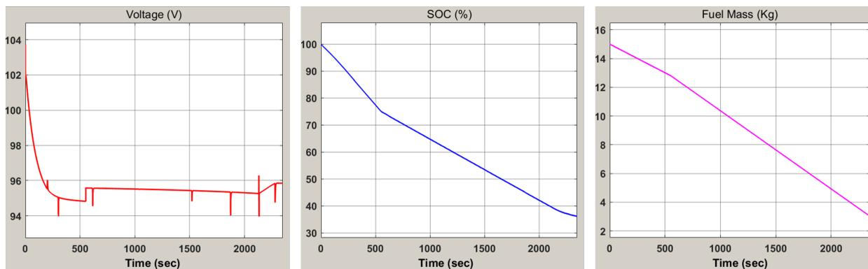
Figure 15: Results of series hybrid - voltage, SOC, fuel mass
