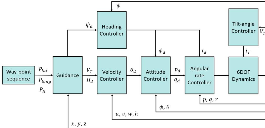
Figure 10: Proposed tiltrotor UAM controller of structure
