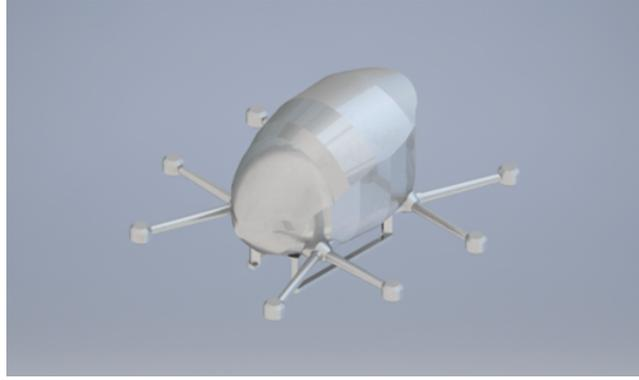
Figure 12: Coaxial octocopter type UAM
