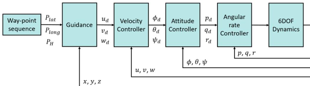
Figure 9: Proposed multirotor UAM controller of structure
