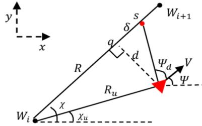
Figure 8: Carrot chasing algorithm variable
