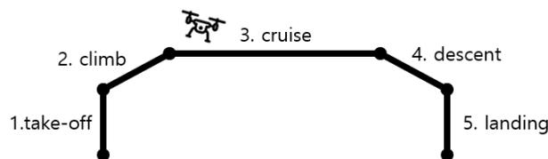
Figure 1: Profile for multirotor type UAM
