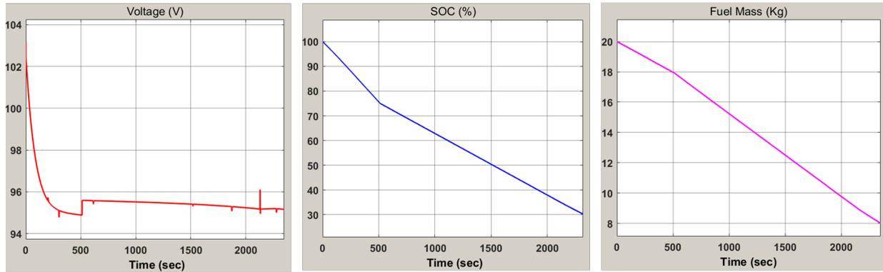
Figure 16: Results of parallel hybrid - voltage, SOC, fuel mass
