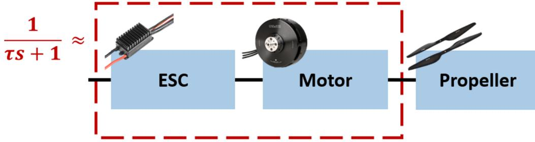
Figure 7: Simplified electric motor model
