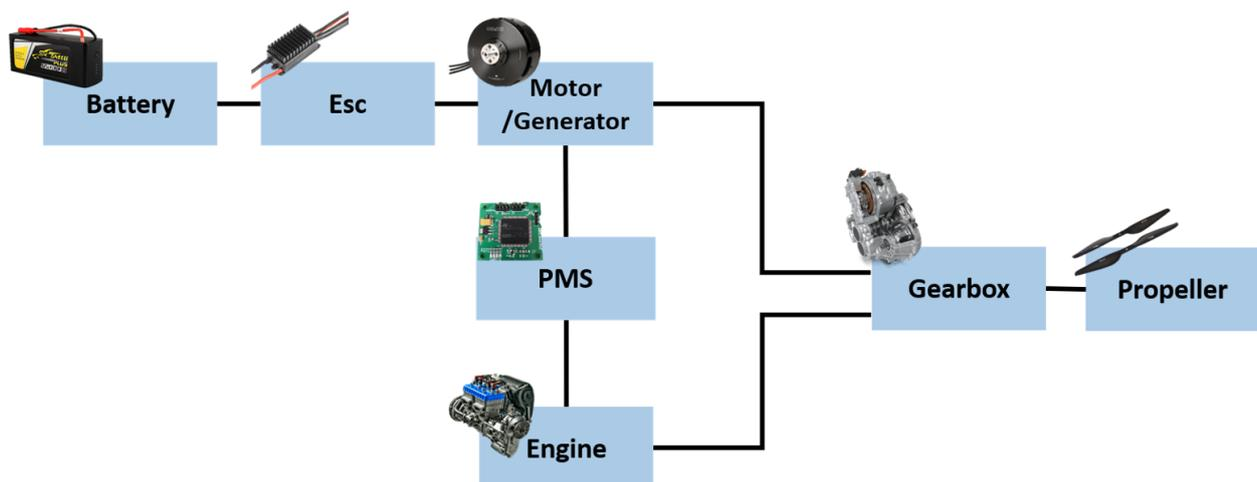
Figure 5: Parallel-hybrid propulsion
