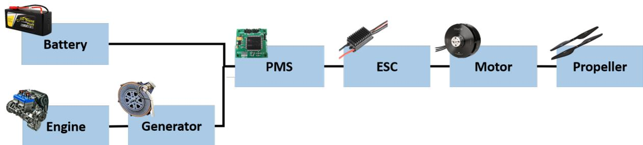
Figure 4: Series-hybrid propulsion
