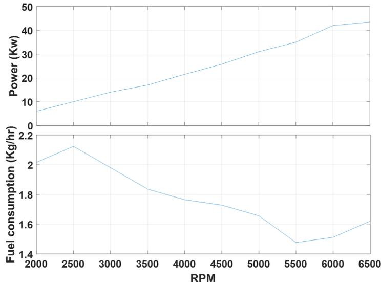
Figure 6: Performance experimental data for DLE 40
