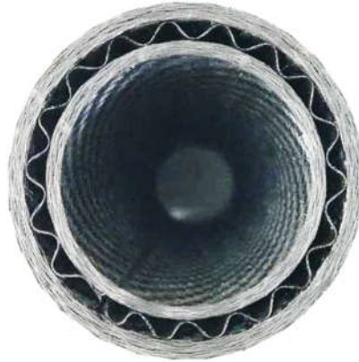
Figure 9 Demonstrator of an internally cooled C/C-SiC tube ( \varnothing 40 mm / \varnothing 56 mm x 175 mm) based on liquid silicon infiltration (LSI) and in situ joining technology.
