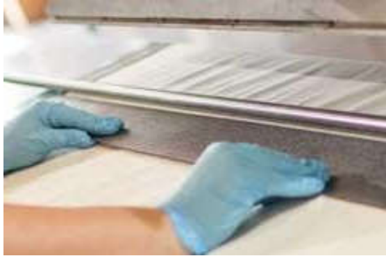
Figure 1 Manufacture of CFRP tubes via prepreg wrapping (left) and wet filament winding (right)
