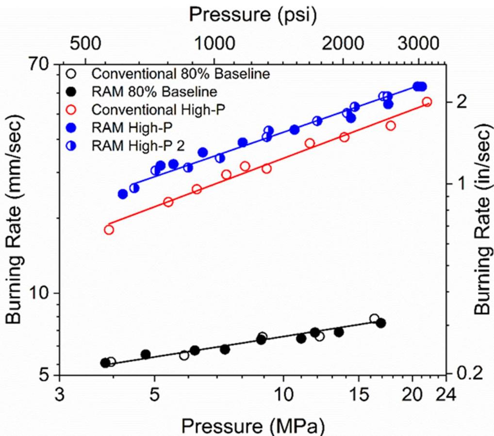
Figure 2. Burning rate data for baseline and high-performance propellant formulations mixed by conventional and RAM methods.
