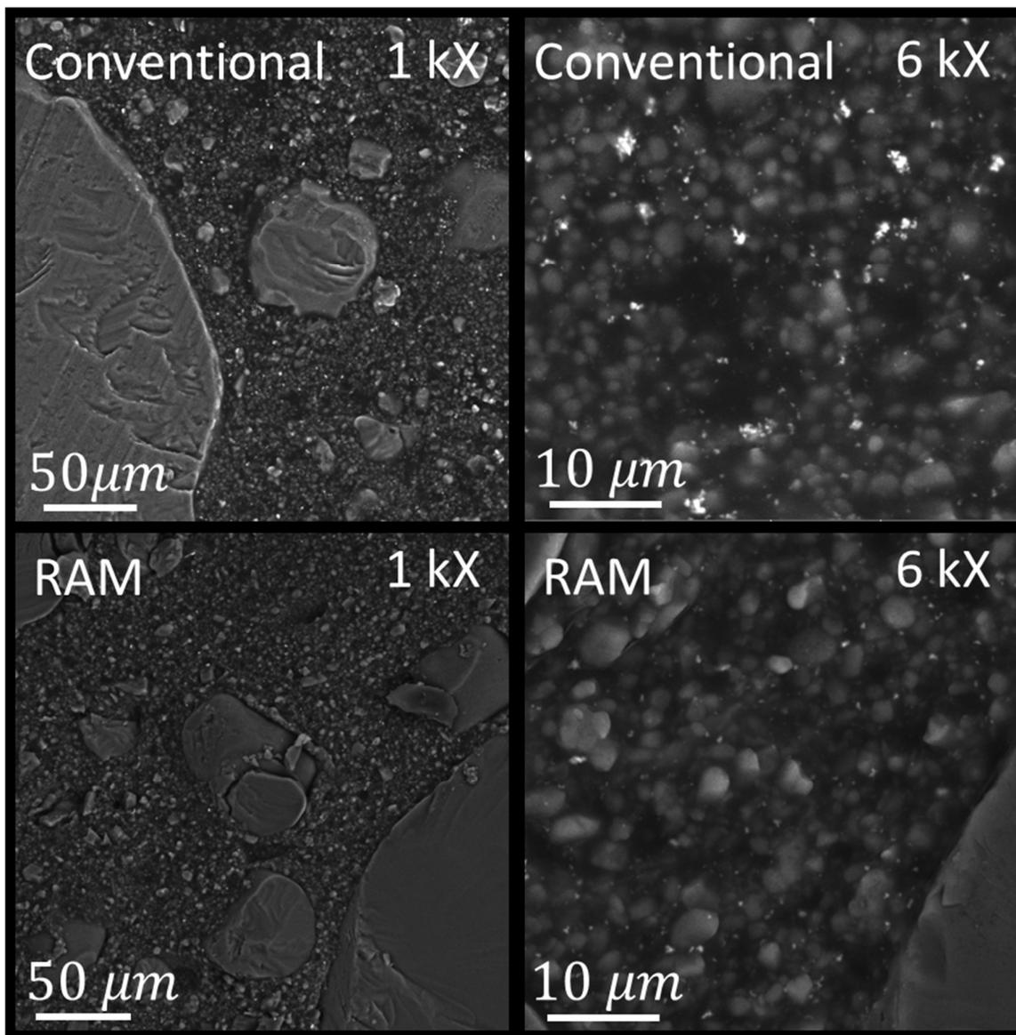
Figure 3. SEM imaging of (top) conventionally mixed and (bottom) RAM propellant samples at (left) 1 kX and (right) 6 kX.
