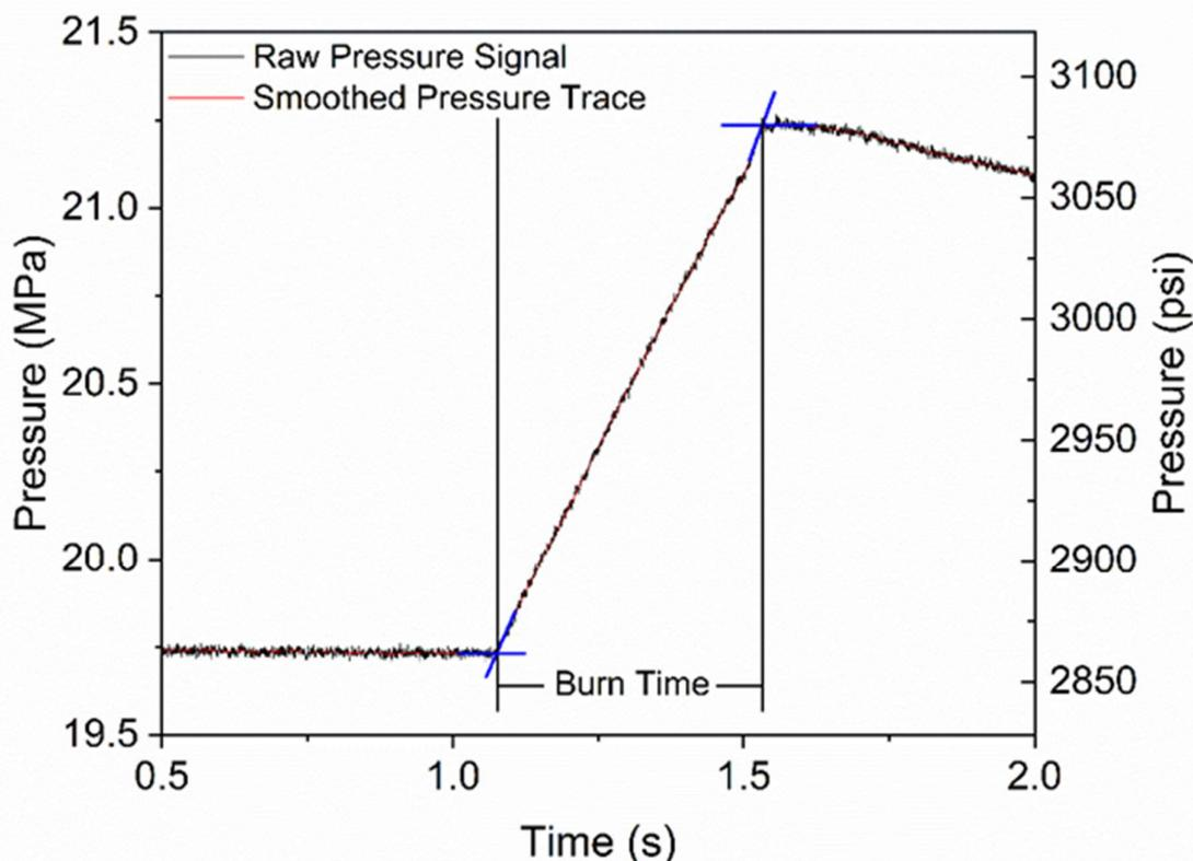
Figure 1. Representative pressure trace from a composite propellant ballistic experiment with the corresponding burn time measurement.
