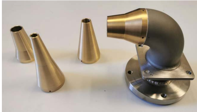
Figure 5. Primary nozzle with the nominal cone and the three different adaptive cones.
