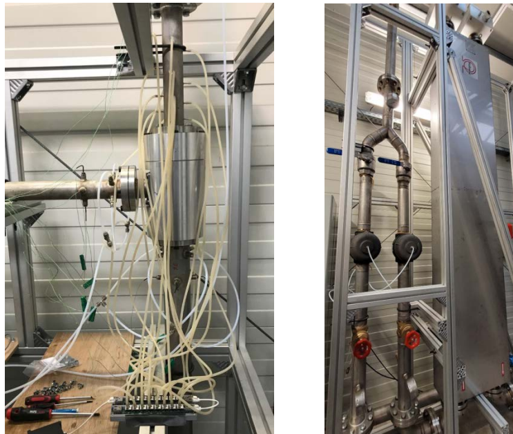
Figure 4: Left: instrumented ejector in the experimental set-up. Right: electrical heater.
