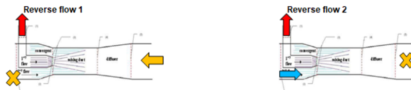
Figure 2: Reverse flow modes during ejector operation.
