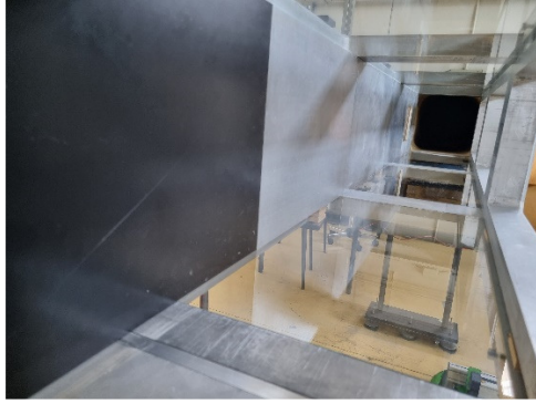
(a) Smooth configuration: Aluminium flat plate
