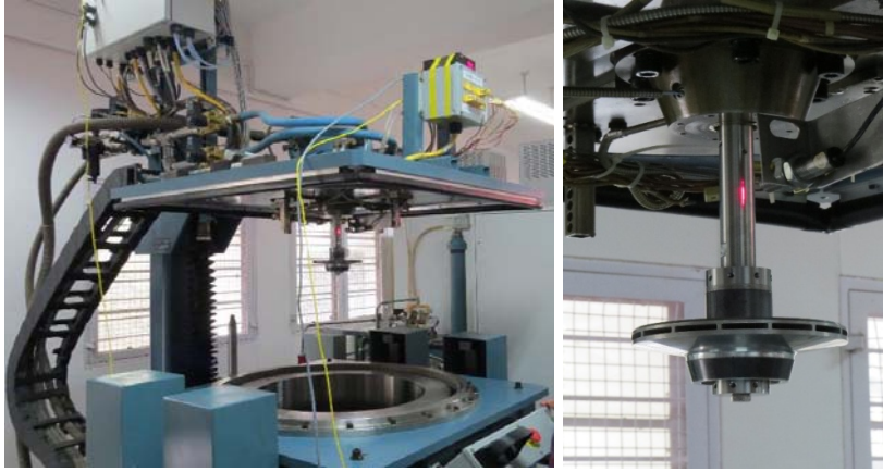
Figure 5 Spin testing of PREBURNER PUMP Impeller
