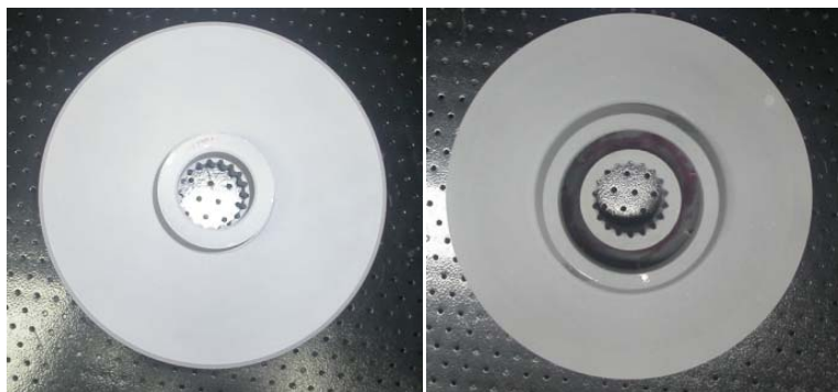
Figure 2: DP test of PREBURNER PUMP Impeller
