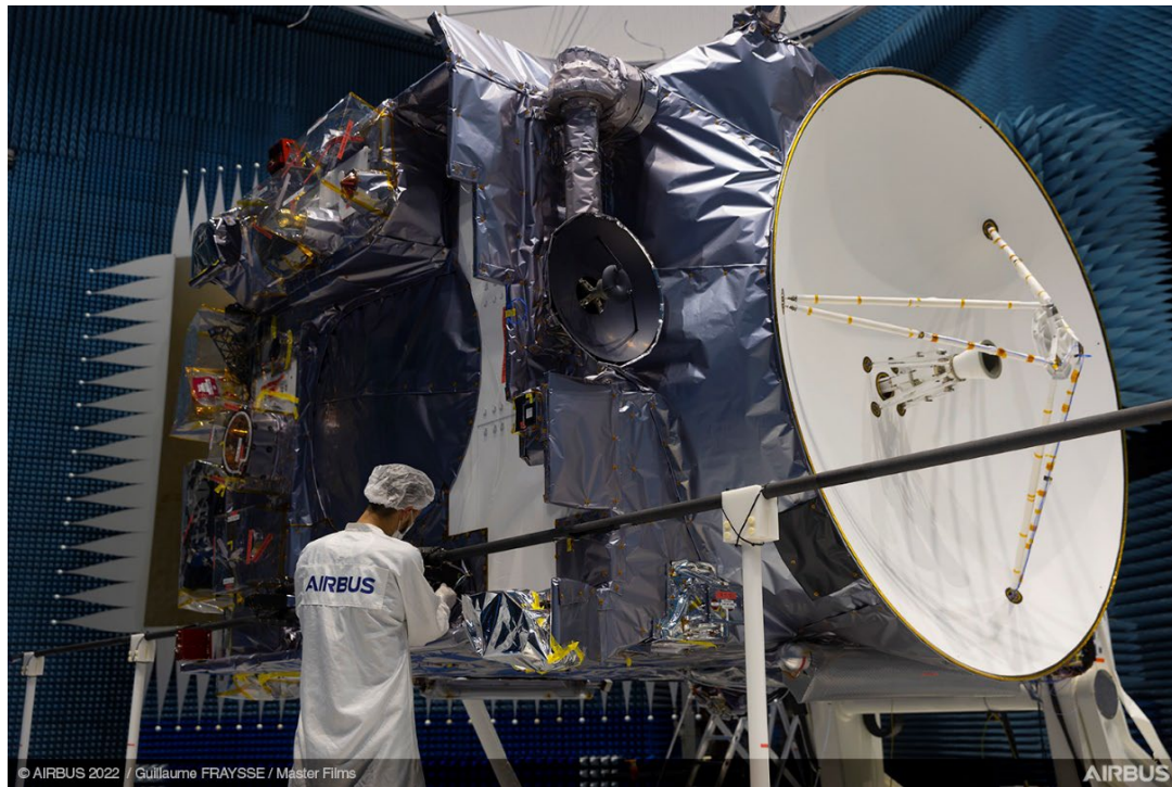
Figure 6: JUICE during the electromagnetic compatibility test (Airbus Toulouse, April 2022)
