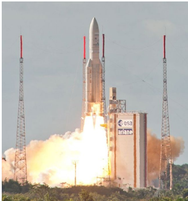
Figure 6 : Four lightning masts surrounding Ariane 5 at launch pad
