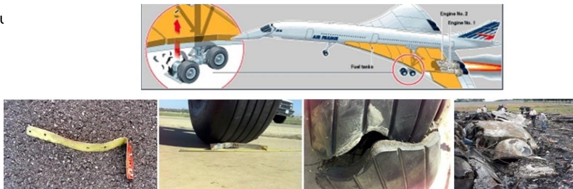
Figures 1-2: Tyre debris object on aircraft wing lower cover observed in service The example of Concorde
