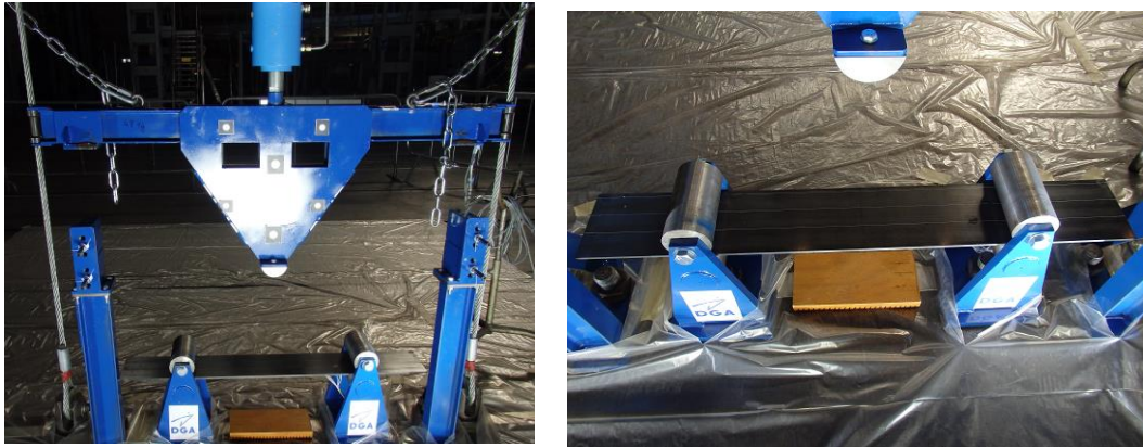
Figures 4-11: Pseudo dynamic tests on stiffened panels – Real test setup and specimen description
