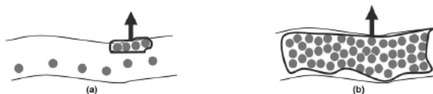
Figure 1: Accumulation of aluminum particles within the mobile layer at ignition. In (a), the layer is partly filled, resulting in a small agglomerate. In (b), the mobile layer is fully saturated, resulting in a large agglomerate [1]
