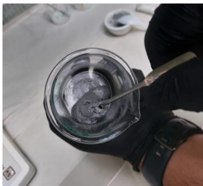
Figure 4: Mixing process of the AP/HTPB/Al solid propellant composition
