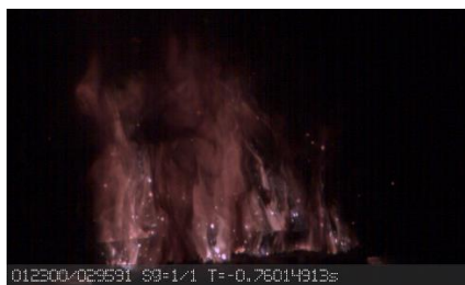
Figure 8: A typical image of the propellant combustion process taken with Chronos 2.1 camera at 5400 frames per second. The photographed strand includes only micro-Al powder and burns at a pressure of 4 MPa
