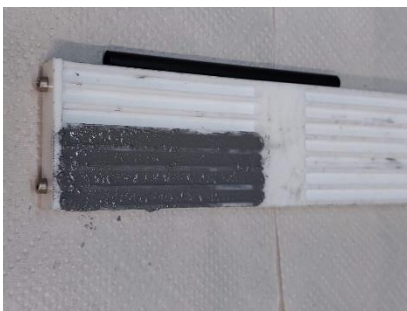
Figure 5: Propellant mixture casted into the mold
