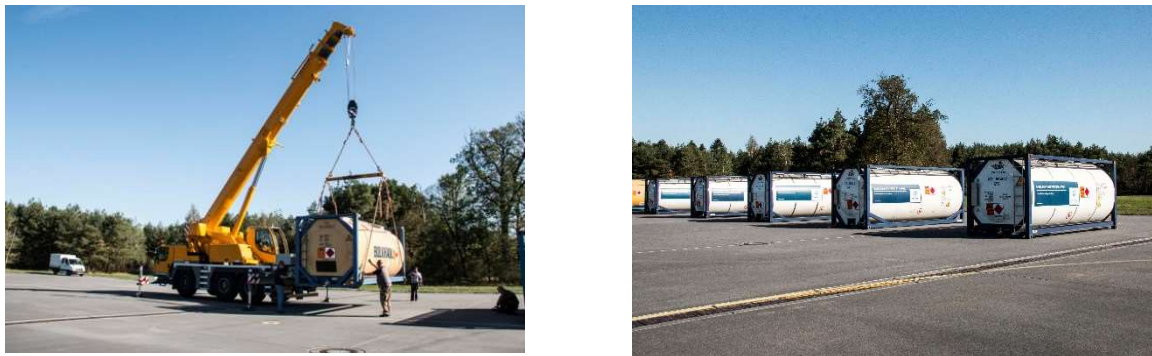
Figure 3: ECLIF1 fuel iso-container delivery and unloading with crane (left). Iso-containers storage in certified dedicated area.
