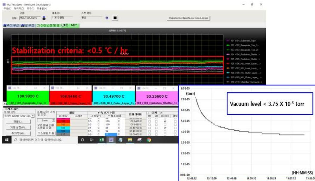
Figure 7: Temperature stabilization and vacuum level criteria
