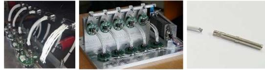
***Figure 8 : Left to right: different harness configurations; modified test rig for shaker operation; broken wire***
