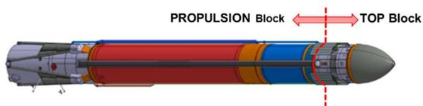
Figure 4: Vehicle TOP Block vs. Propulsion Block
