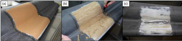
**Figure 10 : Bonded Cork Sheet, (a) after bonding, (b) during removal, (c) after sanding**
