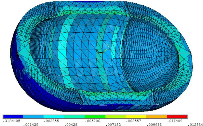
Figure 13: Strain Distribution for 50% Loading
