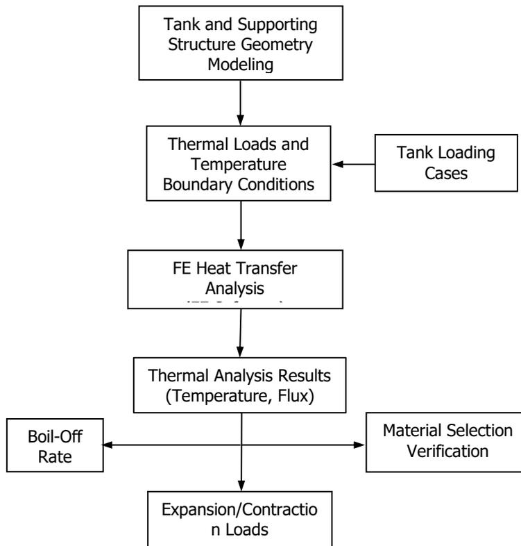
Figure 5: FE Thermal Analysis Process
