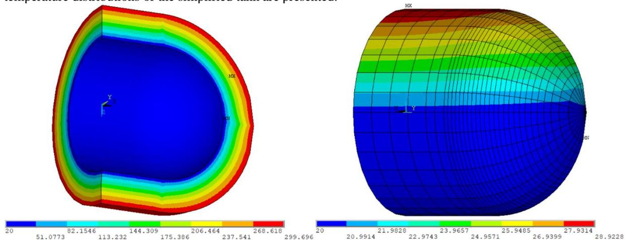
Figure 8 : Temperature Distributions of the entire Tank for 100% loading (left) and of the Inner Tank for 50% loading (right) (units in K)
