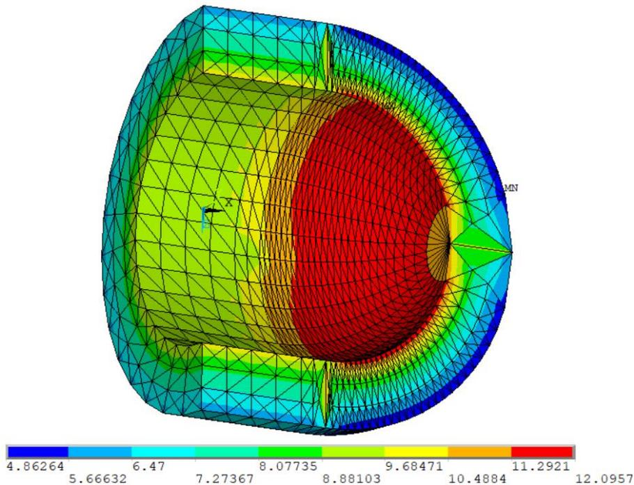
Figure 9: Thermal Flux Distribution of the Modeled Tank (units in  $\text{W/m}^2$ )
