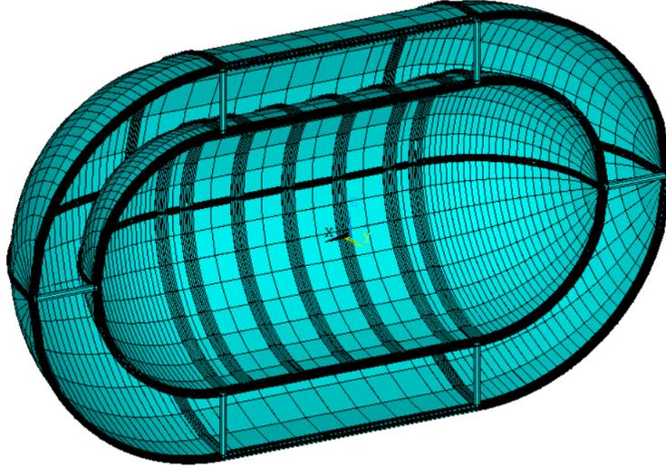
Figure 2: Section of the Modeled Tank Showing the Tank Walls and the Supporting Structure
