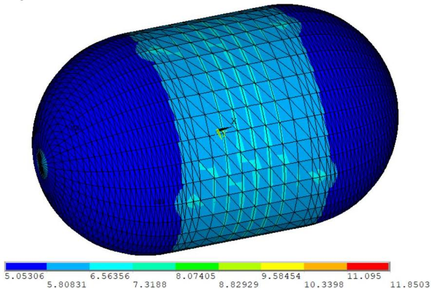
Figure 10: Thermal Flux Distribution on the Outer Tank (units in  $\text{W/m}^2$ )
