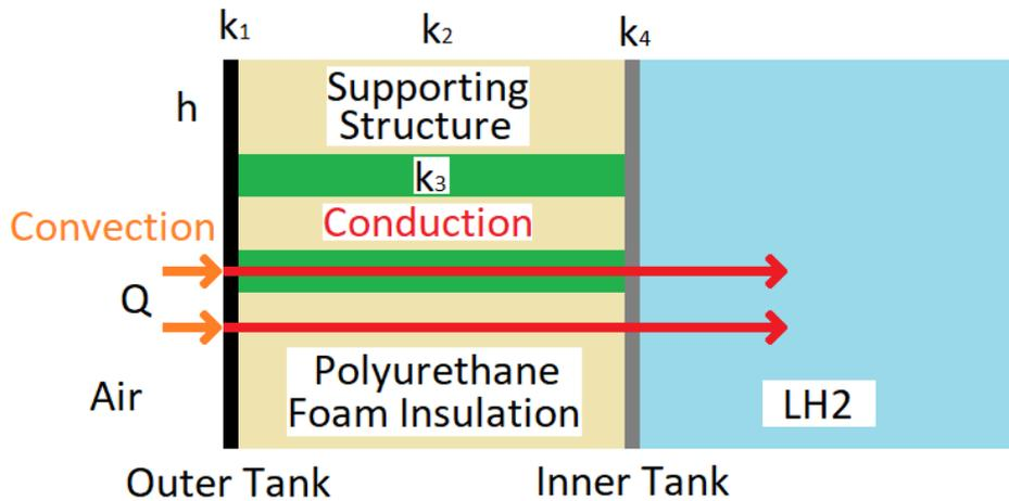
Figure 3: Simplified Analytical Heat Transfer Model for the cryogenic Tank
