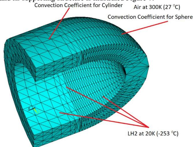
Figure 6: Convection and Temperature Boundary Conditions
