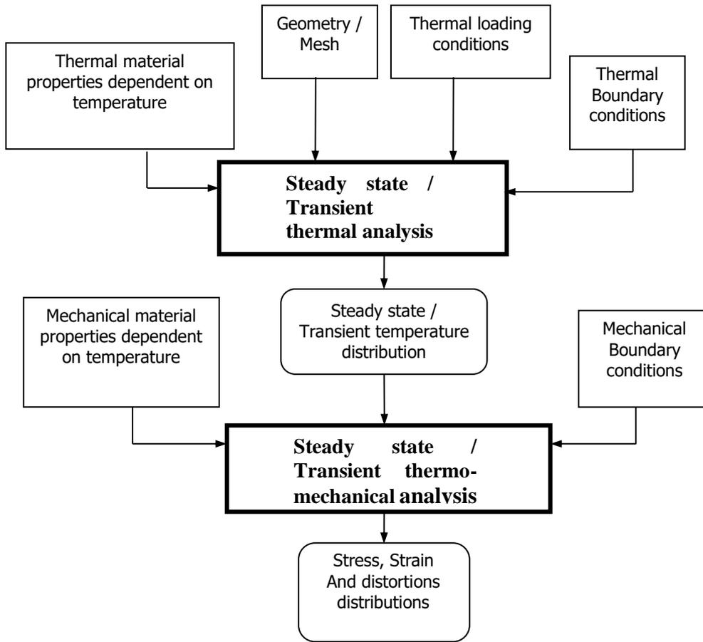
Figure 4: Overview of the thermo-mechanical hydrogen tank simulation
