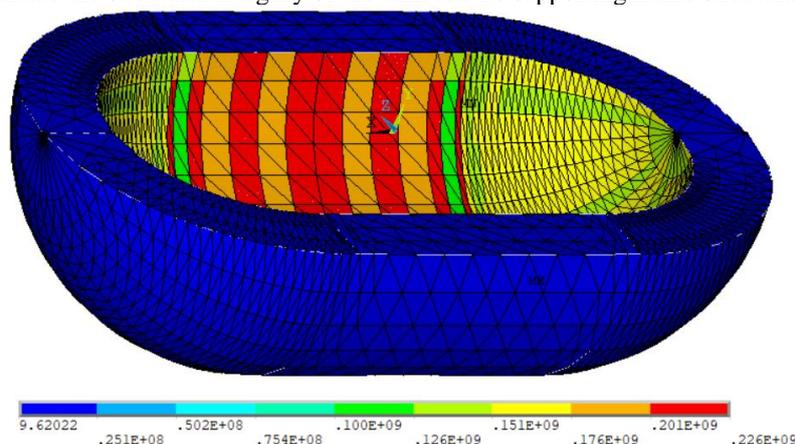
Figure 12: Stress Distribution for 100% Loading [units in Pa]
