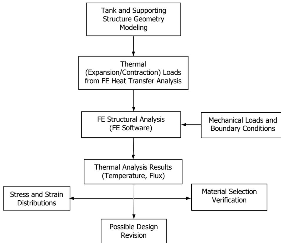
Figure 11 : FE Structural Analysis Process
