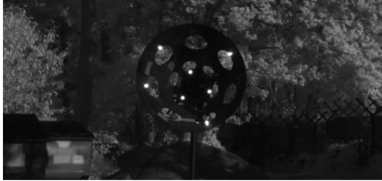
Figure 15: NIR-LED pattern, visible in the cone of the ACCD in static camera tests
