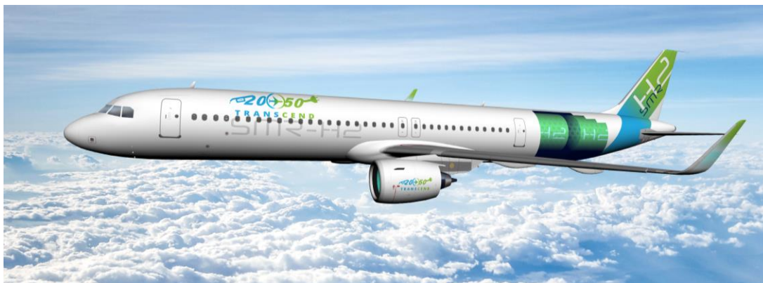
Figure 8: Artist impression of SMR single aisle \text{H}_2 -powered configuration, showing the \text{LH}_2 tanks (aft of the cabin) and fuselage extension.
