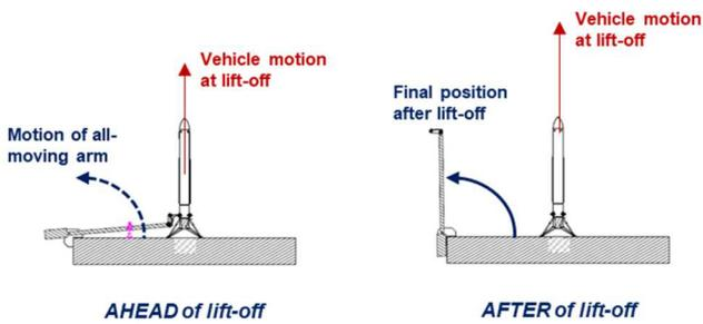
Figure 11 : all-moving arm for supplying gas and electrical power to Vehicle at lift-off pad
