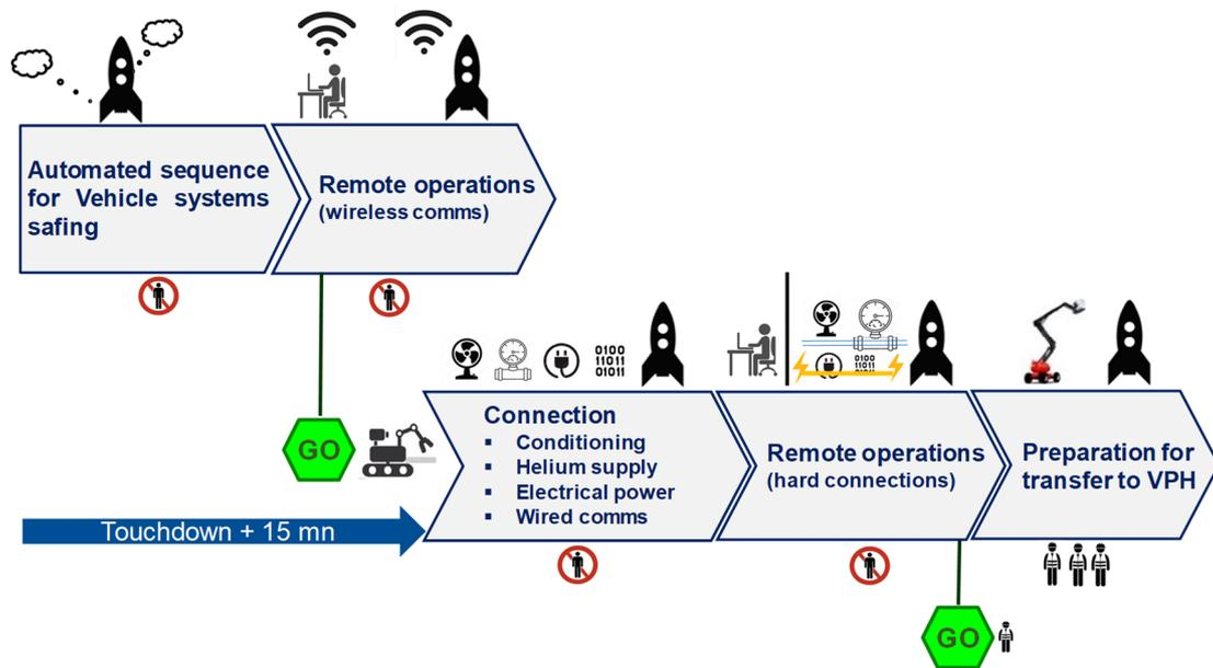
Figure 10 : set of primary operations after landing – scenario relying on robot for reconnections
