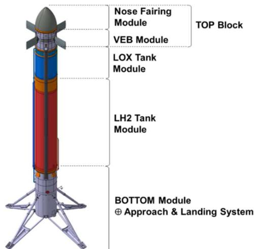
Figure 4: Vehicle configuration
