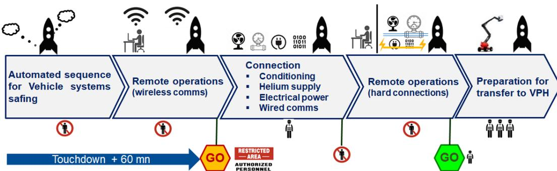
Figure 9 : set of primary operations after landing – scenario relying on staff for reconnections
