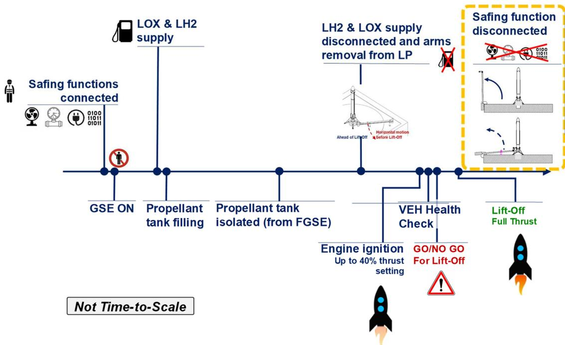
Figure 12: operations at Lift-Off Pad – scenario relying on MGSE disconnected AFTER Vehicle starting to move (vertical motion)
