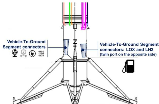
Figure 5: Vehicle-To-Ground Segment interfaces at Lift-Off Pad/Landing Zone
