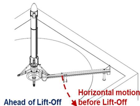
Figure 3 : All-moving cryogenic arm(s) at Lift-Off Pad
