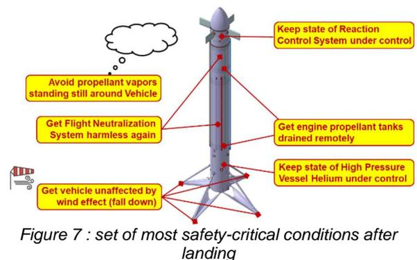
Figure 7 : set of most safety-critical conditions after landing
