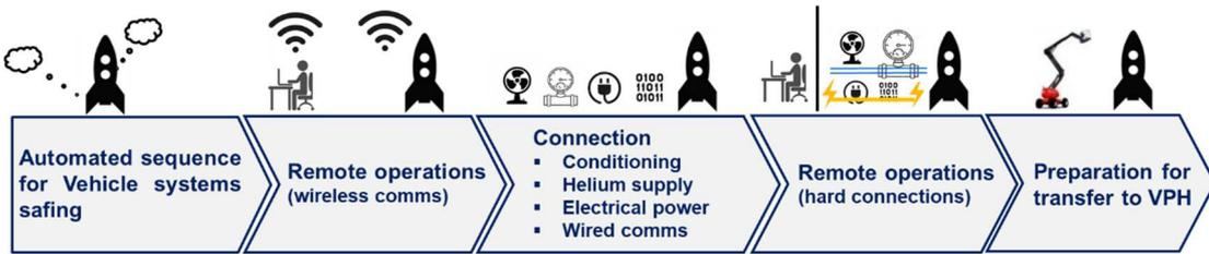
Figure 8 : set of primary operations after landing
