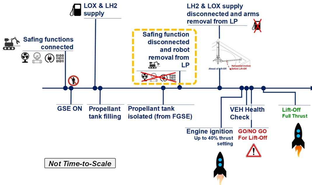
Figure 13: operations at Lift-Off Pad – scenario relying on robot disconnected PRIOR TO Vehicle starting to move (vertical motion)
