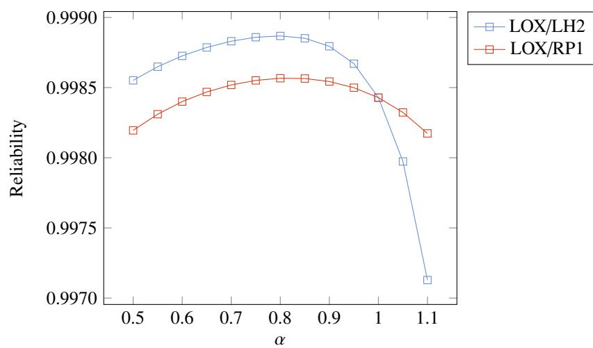
Figure 5: Reliability as function of the de-rating factor  $\alpha$  for different propellant combinations with a constant operational thrust.
