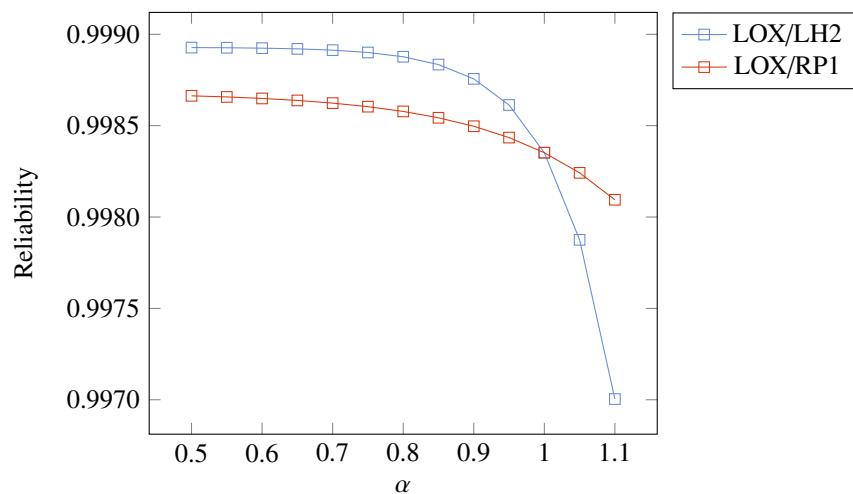
Figure 4: Reliability as function of the de-rating factor  $\alpha$  for different propellant combinations with a constant nominal thrust  $T_{nom}$ .
