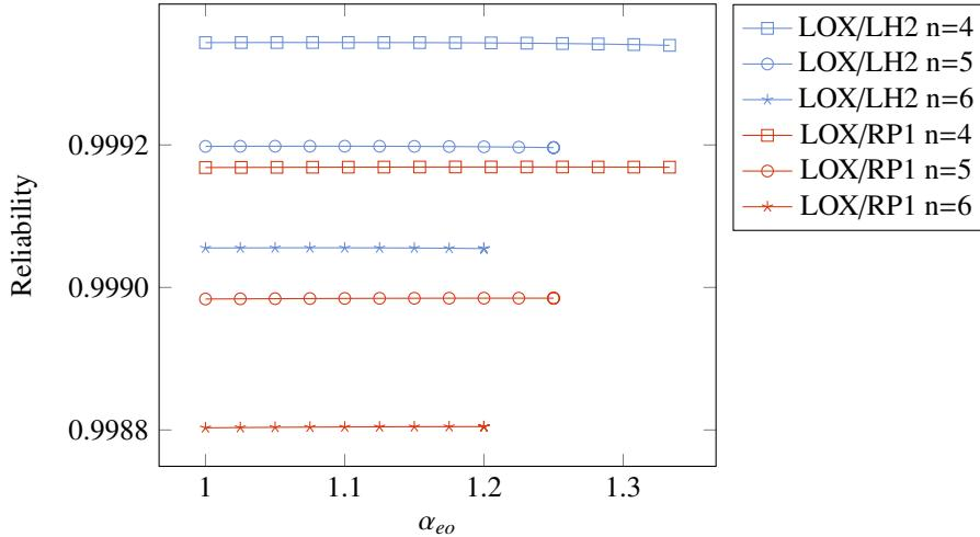
Figure 8: Reliability of a propulsion system with engine out capability as function of  $\alpha_{eo}$  for a different number of engines and different propellant combinations. An initial de-rating factor of  $\alpha = 0.8$  was considered in all cases.
