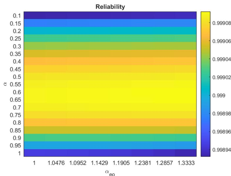
Figure 10: Heatmap showing the reliability as a function of  $\alpha$  and  $\alpha_{eo}$ , for  $0.1 \leq \alpha \leq 1$  and  $1 \leq \alpha_{eo} \leq 1.333$ . The configuration with 4 engines providing  $2278 \text{ kN}$  of operational thrust for a  $500 \text{ s}$  burn using DBFRSC cycle was used.
