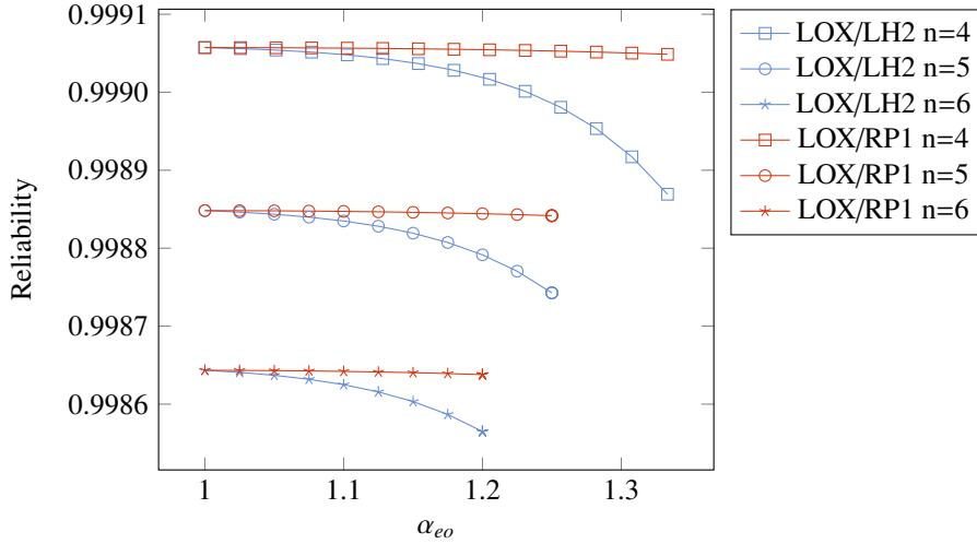
Figure 7: Reliability of a propulsion system with engine out capability as function of  $\alpha_{eo}$  for a different number of engines and different propellant combinations. An initial de-rating factor of  $\alpha = 1$  was considered in all cases.
