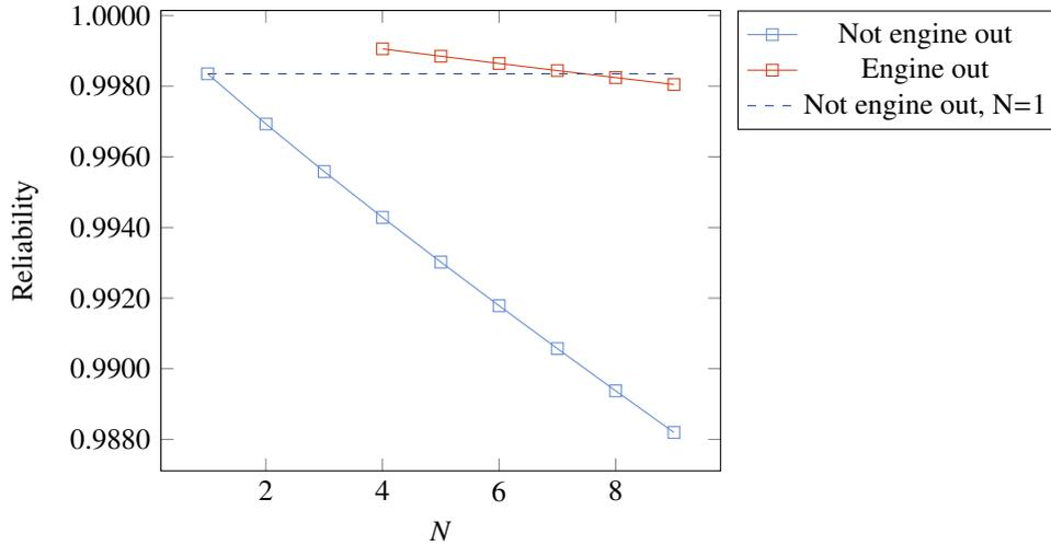
Figure 6: Reliability as a function of the number of engines, for engine out capability and not engine out capability, assuming DBFRSC engine cycle using LOX/LH2 with  $T = 2278kN$  for a 500 s burn, with  $\alpha = 1$  and  $\alpha_{eo} = 1$ . The dashed line represents the reliability using only one engine to be used as a reference for comparison with the engine out case.
