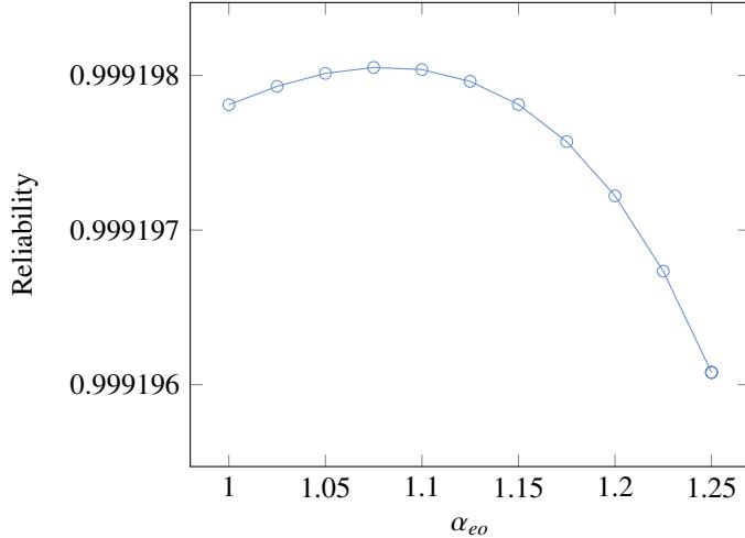
Figure 9: Reliability of a propulsion system with engine out capability as function of  $\alpha_{eo}$  for a different number of engines and different propellant combinations. An initial de-rating factor of  $\alpha = 0.8$  was considered.
