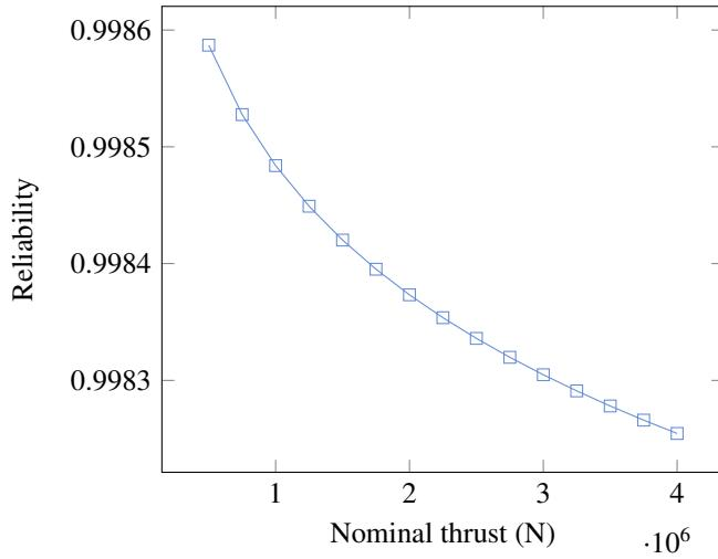
Figure 2: Reliability as a function of the nominal thrust, assuming DBFRSC engine cycle using LOX/LH2 and 500 s burn.
