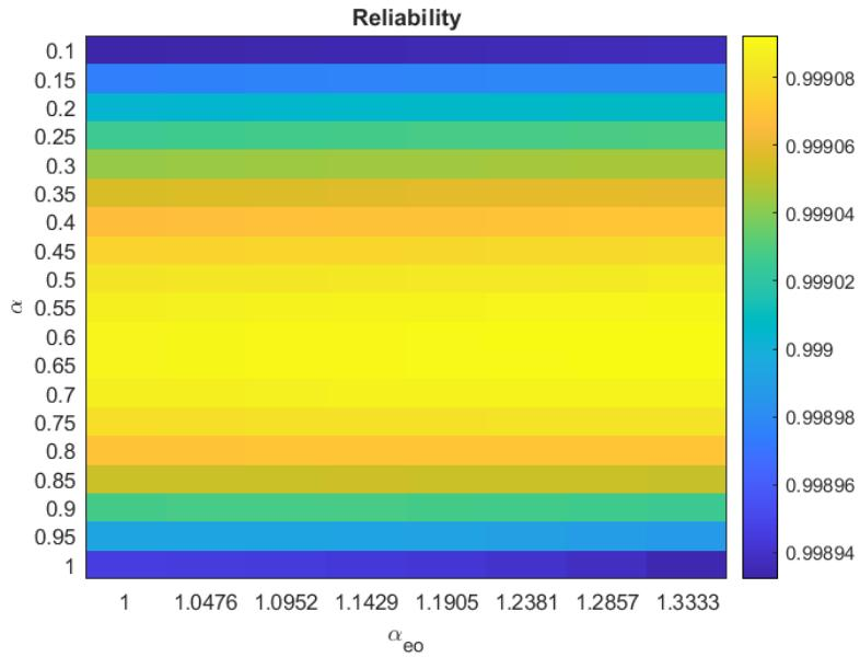
Figure 10: Heatmap showing the reliability as a function of  $\alpha$  and  $\alpha_{eo}$ , for  $0.1 \leq \alpha \leq 1$  and  $1 \leq \alpha_{eo} \leq 1.333$ . The configuration with 4 engines providing 2278kN of operational thrust for a 500s burn using DBFRSC cycle was used.
