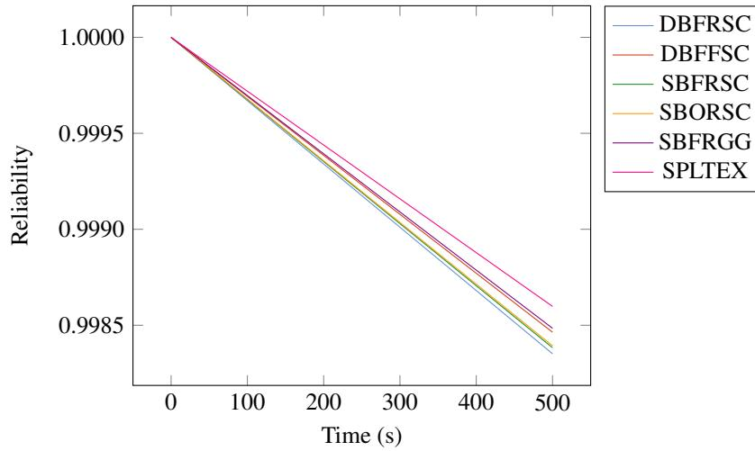
Figure 1: Reliability as a function of time for different engine cycles.
