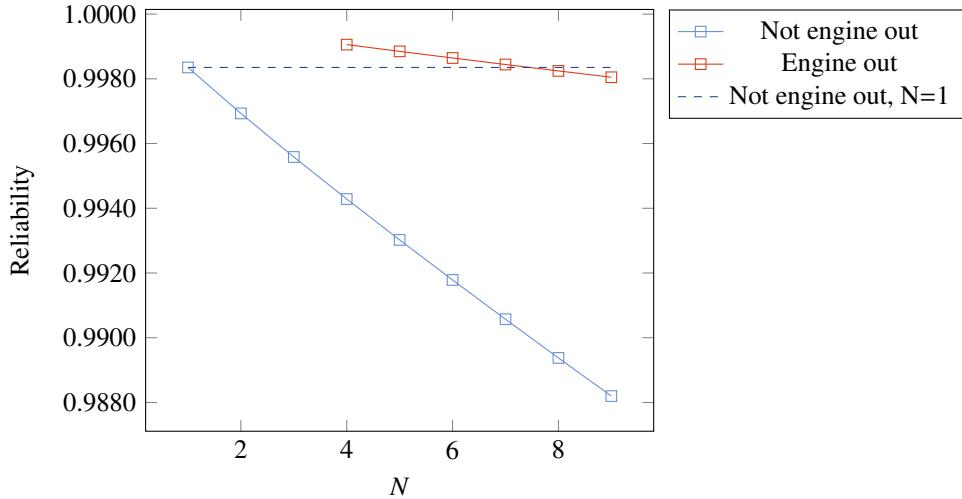
Figure 6: Reliability as a function of the number of engines, for engine out capability and not engine out capability, assuming DBFRSC engine cycle using LOX/LH<sub>2</sub> with  $T = 2278\text{kN}$  for a 500 s burn, with  $\alpha = 1$  and  $\alpha_{eo} = 1$ . The dashed line represents the reliability using only one engine to be used as a reference for comparison with the engine out case.
