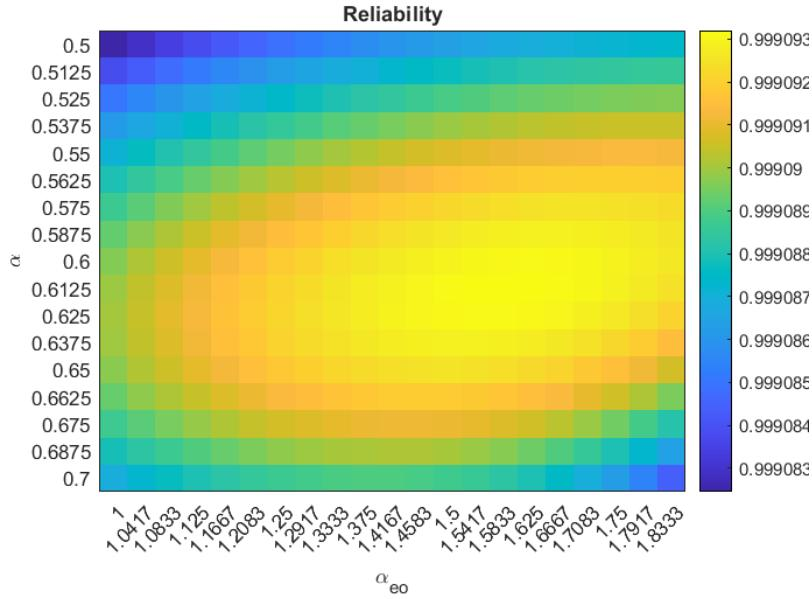
Figure 11: Heatmap showing the reliability as a function of  $\alpha$  and  $\alpha_{eo}$ , for  $0.5 \leq \alpha \leq 0.7$  and  $1 \leq \alpha_{eo} \leq 1.833$ . The configuration with 4 engines providing  $2278\text{kN}$  of operational thrust for a 500s burn using DBFRSC cycle was used.
