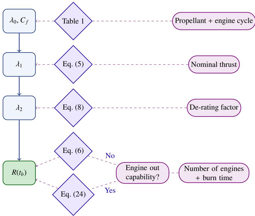
Figure 13: Process followed to calculate the reliability of the propulsion system.
