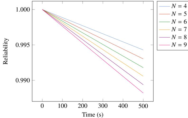
Figure 3: Reliability as a function of time for different number of engines, assuming DBFRSC engine cycle using LOX/LH2 and 500 s burn.
