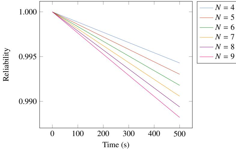
Figure 3: Reliability as a function of time for different number of engines, assuming DBFRSC engine cycle using LOX/LH<sub>2</sub> and 500 s burn.
