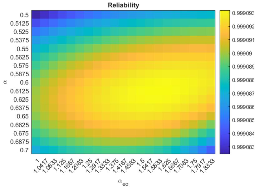
Figure 11: Heatmap showing the reliability as a function of  $\alpha$  and  $\alpha_{eo}$ , for  $0.5 \leq \alpha \leq 0.7$  and  $1 \leq \alpha_{eo} \leq 1.833$ . The configuration with 4 engines providing  $2278kN$  of operational thrust for a  $500s$  burn using DBFRSC cycle was used.
