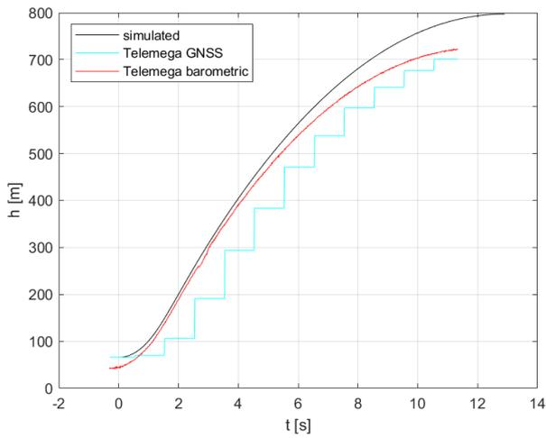
Figure 4: Comparison of altitude for A2e flight
