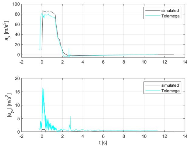
Figure 8: Comparison of accelerations for A2e flight
