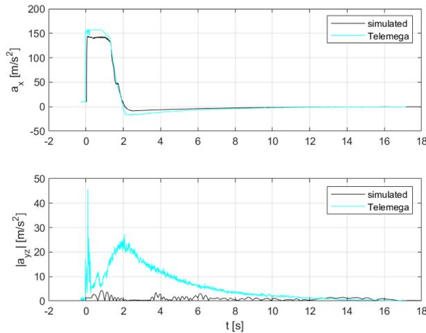
Figure 20: Comparison of acceleration for FOK-1B flight
