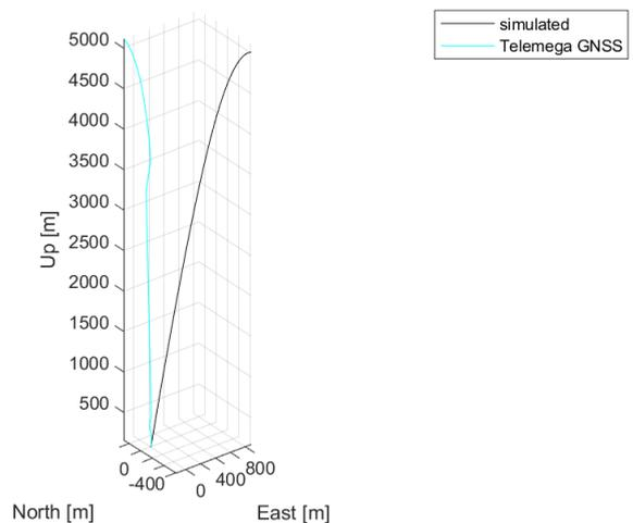
Figure 11: Comparison of 3D trajectory for TuCAN flight
