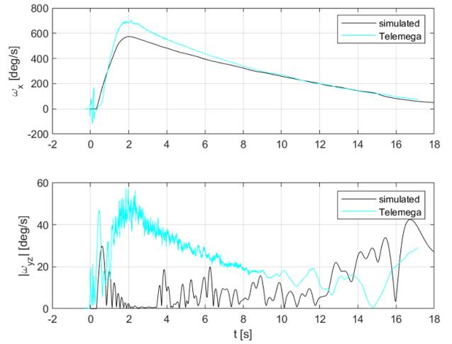
Figure 19: Comparison of angular rates for FOK-1B flight
