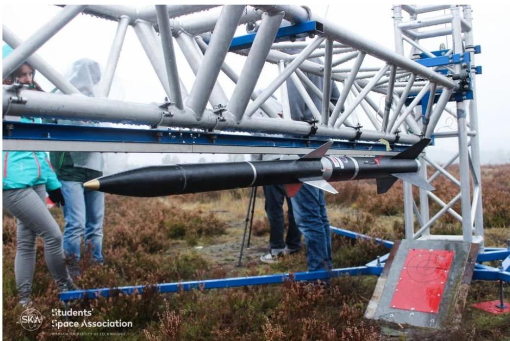
Figure 3: A2 rocket on the launch rail during the rocket launch test
