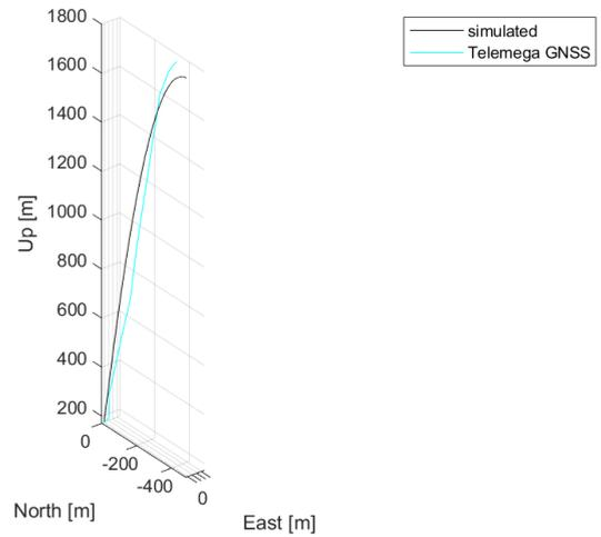
Figure 17: Comparison of 3D trajectory for FOK-1B flight
