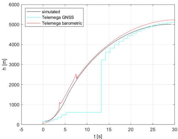
Figure 10: Comparison of altitude for TuCAN flight
