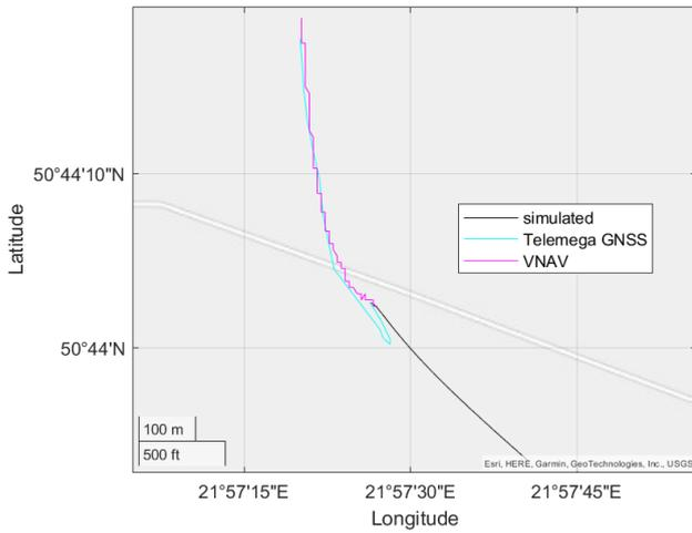
Figure 23: Comparison of geographical coordinates for FOK-1C flight
