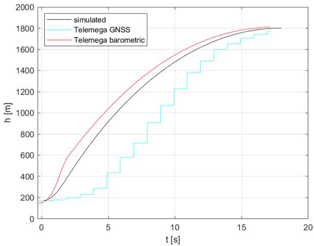
Figure 16: Comparison of altitude for FOK-1B flight
