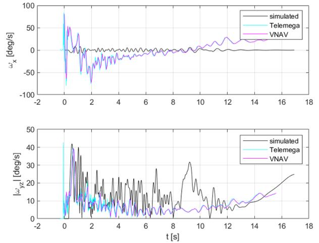
Figure 24: Comparison of angular rates for FOK-1C flight
