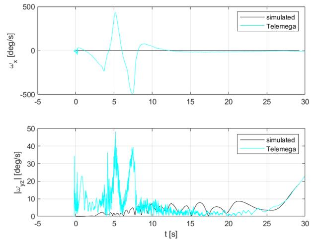
Figure 13: Comparison of angular rates for TuCAN flight
