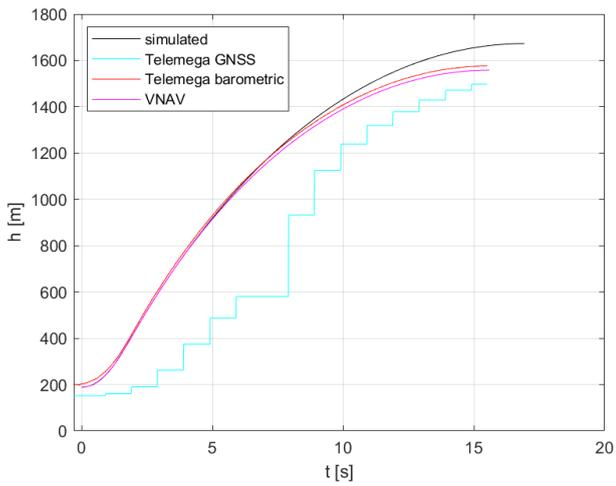
Figure 21: Comparison of altitude for FOK-1C flight
