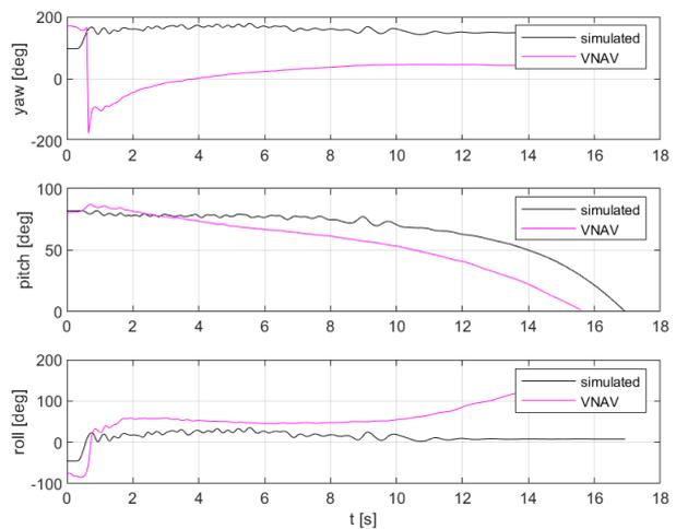
Figure 26: Comparison of attitude angles for FOK-1C flight
