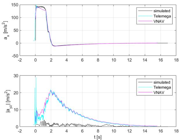
Figure 25: Comparison of acceleration for FOK-1C flight
