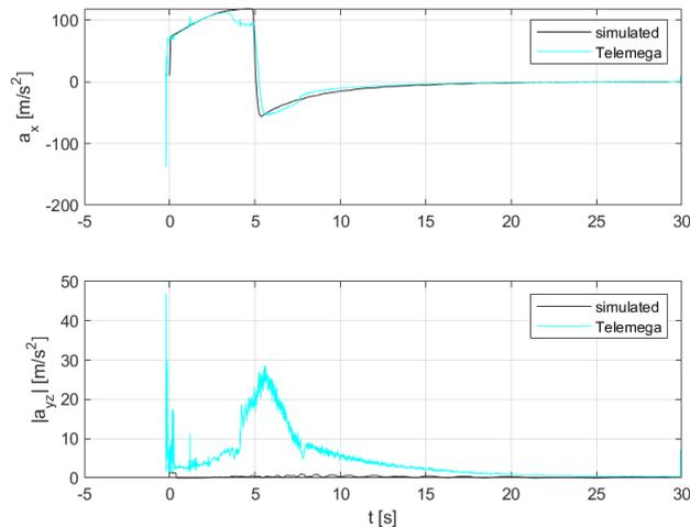
Figure 14: Comparison of acceleration for TuCAN flight
